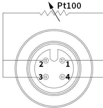
The OM-CP-HITEMP140-M12 is compatible with probes that have the wiring configuration as shown to the left.
