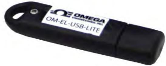
This low cost data logger measures and stores up to 4,080 temperature readings over a -10 to +50 °C (+14 to +122 °F) measurement range with a fixed 30 minute sample rate and a battery life of 1 month continuous use.
