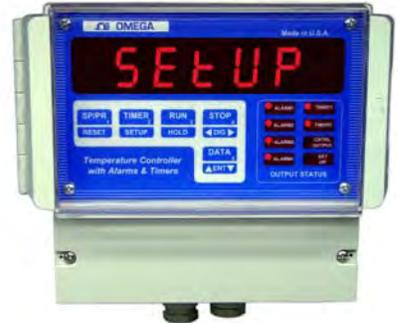
To return from **SETUP** to normal display/run mode, simply push and hold down the '**RESET**' key. On exiting, the display will briefly show '**SAVING**' to indicate that the new data is being saved in nonvolatile memory (key should be held in until the word '**SAVING**' shows up on the display). Setup mode is also exited automatically if no key action is detected for about 5 minutes.
