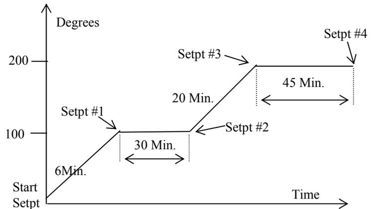
*Figure 2. Example Ramp/Soak profile*
