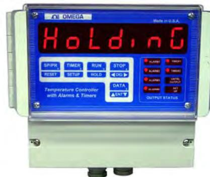
HOLDING or vice versa), the unit will maintain its current status. HOLD mode is also indicated when the run mode indicator (flashing red dot in lower right corner of the display) stops flashing and stays on in steady mode.
