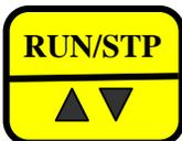
\* This key functions only after a controller has been selected by pushing **CTR. SEL** key. It is used for displaying and changing the current status of selected controller (RUNNING, HOLDING. STOPPED & ENTER SP).
