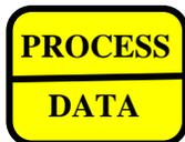
\* Toggling this key will sequentially display process value for each controller. DATA
