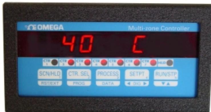
The five CN1500 keys have several functions packed into each key. These Functions are listed below.
