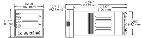
Prior to mounting the CN8500 Series in your panel, make sure that the cutout opening is of the right size, 1.771" x 1.771" (45 mm x 45 mm), and deburred to enable a smooth fit. A minimum of 4" (100 mm) of depth behind the panel is required.
