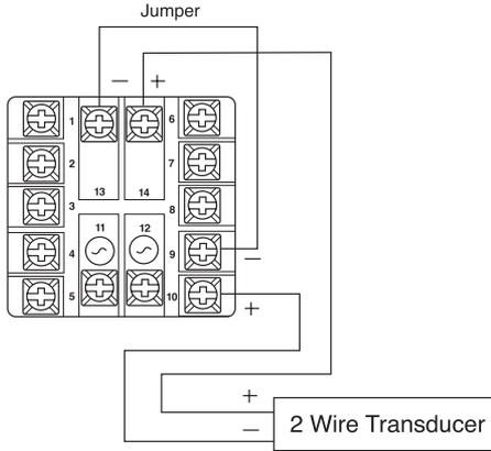
**Figure 15. Wiring Diagram for Transducer Excitation**
