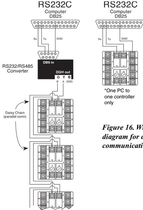
**Figure 16. Wiring diagram for digital communications.**
