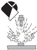
Retaining nuts that may have been in contact with such substances, e.g. due to leakage or spilling, must be replaced.
