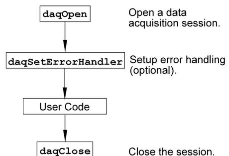
All Visual Basic programs should include the **PDAQX.BAS** file into their project. The **PDAQX.BAS** file provides the necessary definitions and function prototyping for the **DaqX** driver **DLL**.
