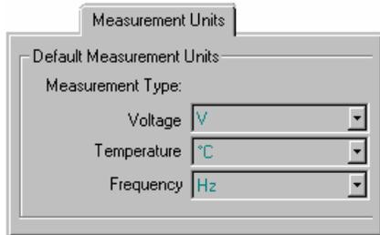
**Measurement Units** – Allows you to set the desired default units for the *Channel Configuration Window's* spreadsheet. Note that scale and offset automatically reset to a pre-designated default according to the unit selected.
