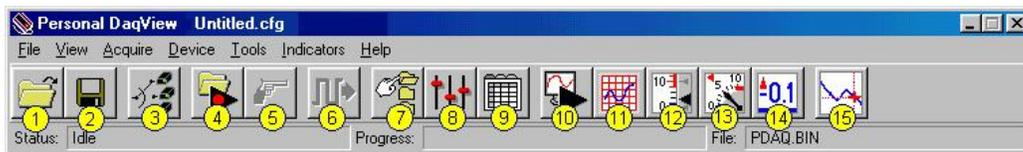
Click one of the toolbar's display icon buttons (11, 12, 13, or 14) to see your data in the form of a chart or meter. Display options are as follows: (11) is scrolling charts, (12) is bar graph meters, (13) is analog meters, and (14) is digital meters. Note that you can view all display types, or a combination of them, at the same time.
