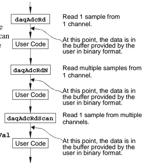
This program will initialize the Personal Daq hardware, then take readings from the analog input channels in the base unit (not the expansion module). For transporting data in and out of the Personal Daq driver, arrays are dimensioned.
