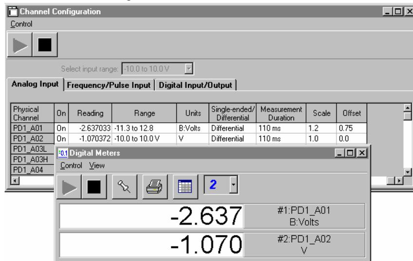
***PD1\_A01 B:Volts Readings resulting from use of the Scale/Offset Feature.
