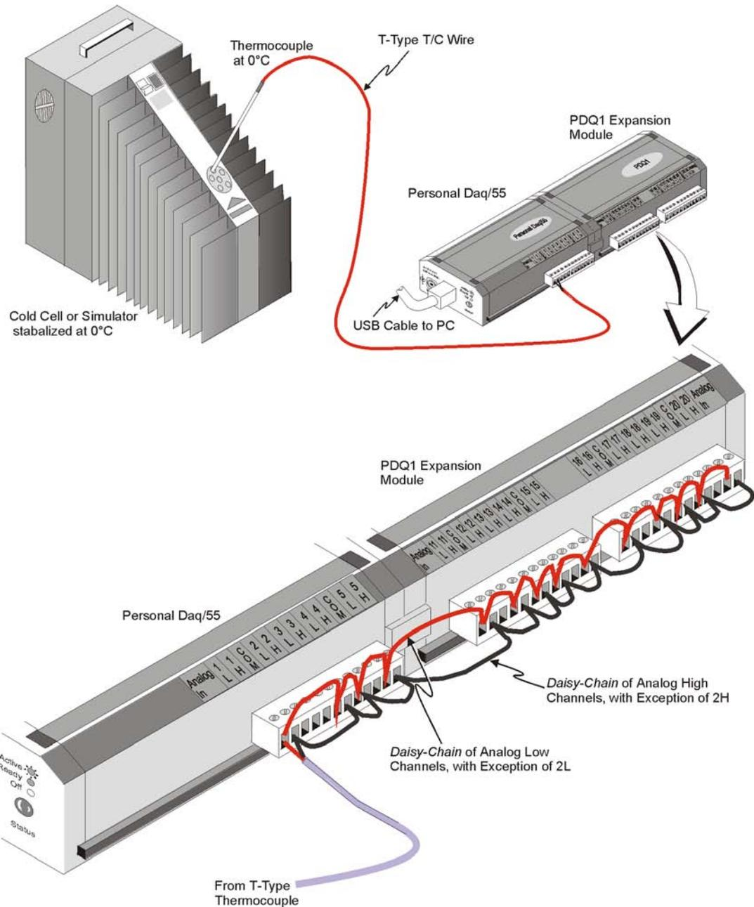
CJC Calibration. Thermocouple is connected with red (-) wire to 1L and blue (+) wire to 1H. Analog Highs and Lows are daisy-chained as indicated. Note that 2L and 2H are left open for voltage-related connections as discussed in step 7.
