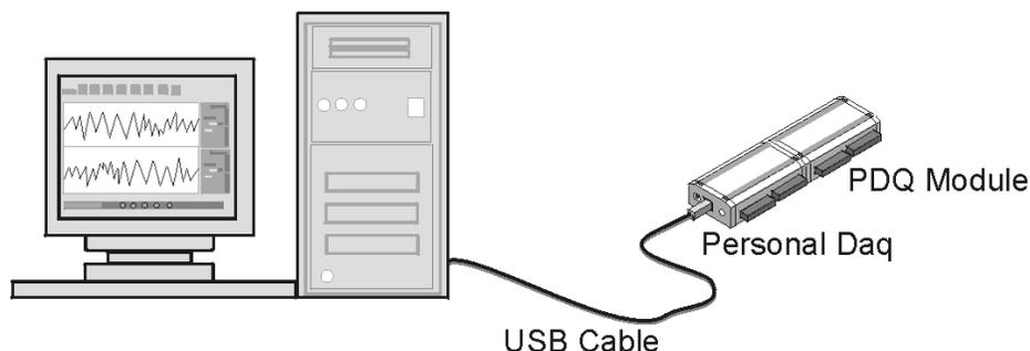
*Connection of a Simple Personal Daq System to a Computer USB Port*
