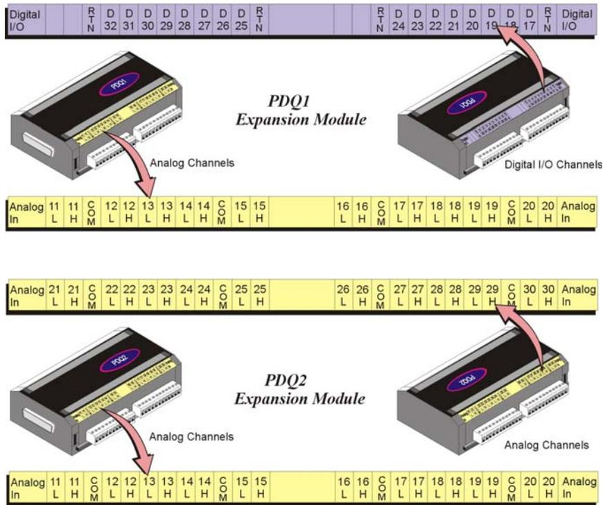
**Digital input** lines can be read as part of the analog scan sequence and can be scanned over 100 times per second. Digital input voltage may range from 0 to +15V, with the logic threshold at <1.3V (low) and >3.8V (high). Digital values outside of the 0 to +15V range are not permitted.
