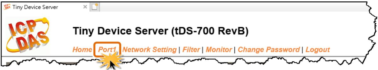
The **Port 1 Settings** section provides functions allowing items such as port settings, serial data packing and pair-connection settings to be configured.
