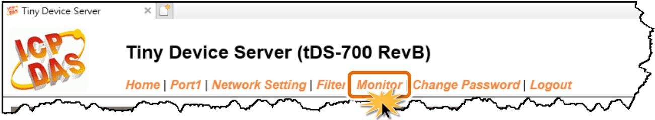
After clicking the **Monitor** tab, the Current Connection Status page will be displayed showing detailed information regarding the current status of the serial port connection settings for the tDS-700 module.
