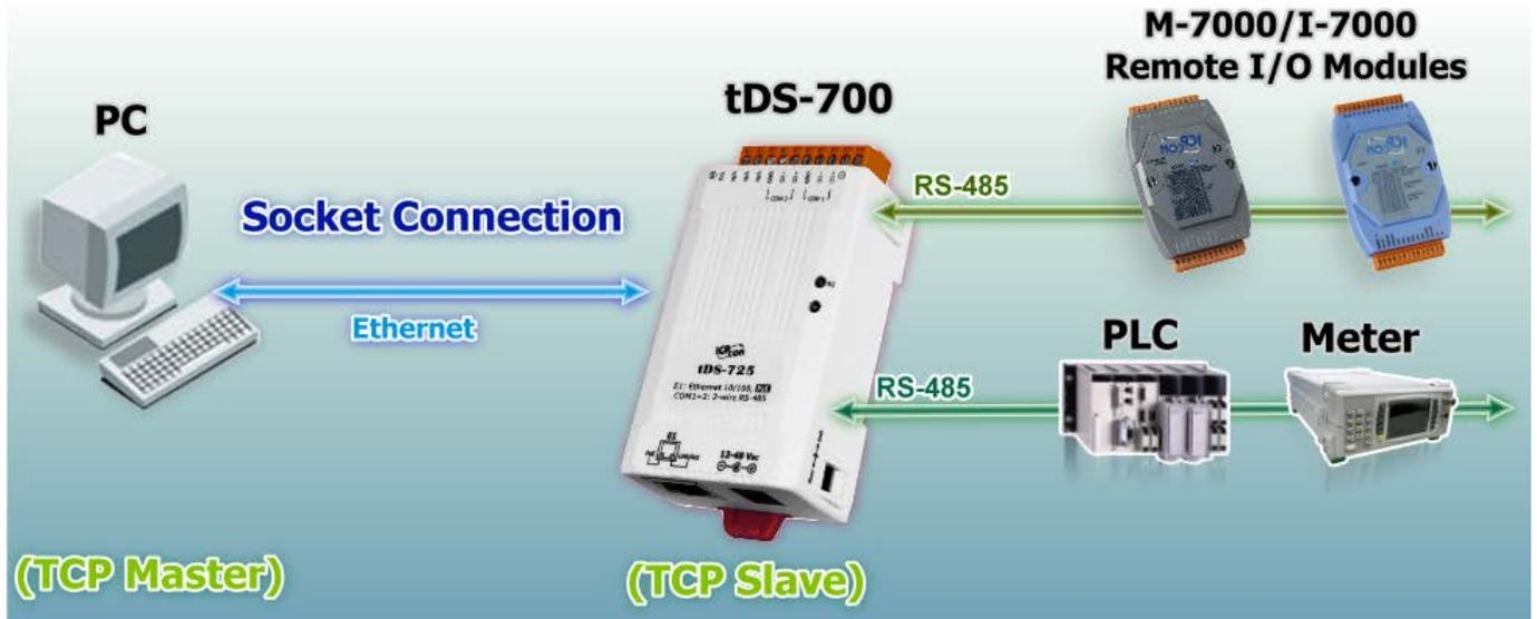
tDS-700 series module can accept the TCP connection (include raw data) directly, it also can communicate with TCP client and Serial Device in this way.
