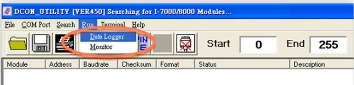
2: Configure the system connection as shown below and click the “Start” button to begin logging data.
