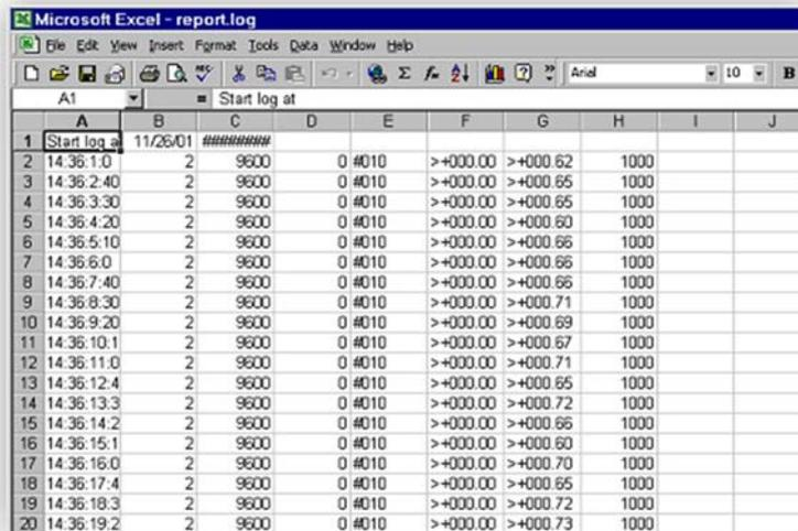
By using the I-7000 DCON utility and MS Excel in conjunction with **VxComm technology**, the signal data originating from I-7000 modules via the Ethernet network can be analyzed without the need to write custom programs. For more information about the **log function**, refer to the online help feature (English and Traditional Chinese) of the DCON utility.
