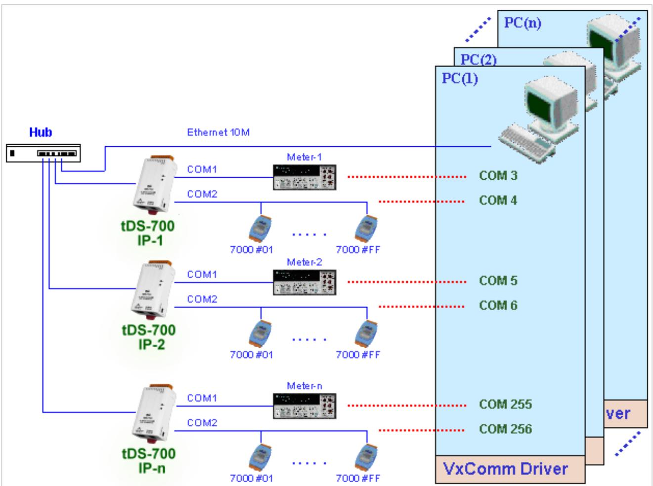
The VxComm driver controls all the details of the Ethernet TCP/IP programming technique, meaning that, with the assistance of tDS-700 and VxComm technology, your COM Port program will be able to access your serial devices through the Ethernet in the same way as through a COM Port.
