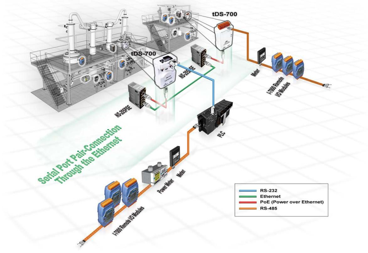
In harsh industrial environments, the tDS-700 series (for i version) also adds 3000 V<sub>DC</sub> and +/- 4 kV ESD protection component that diverts the potentially damaging charge away from sensitive circuit to protect the module and equipment from the sudden and momentary electric current.
