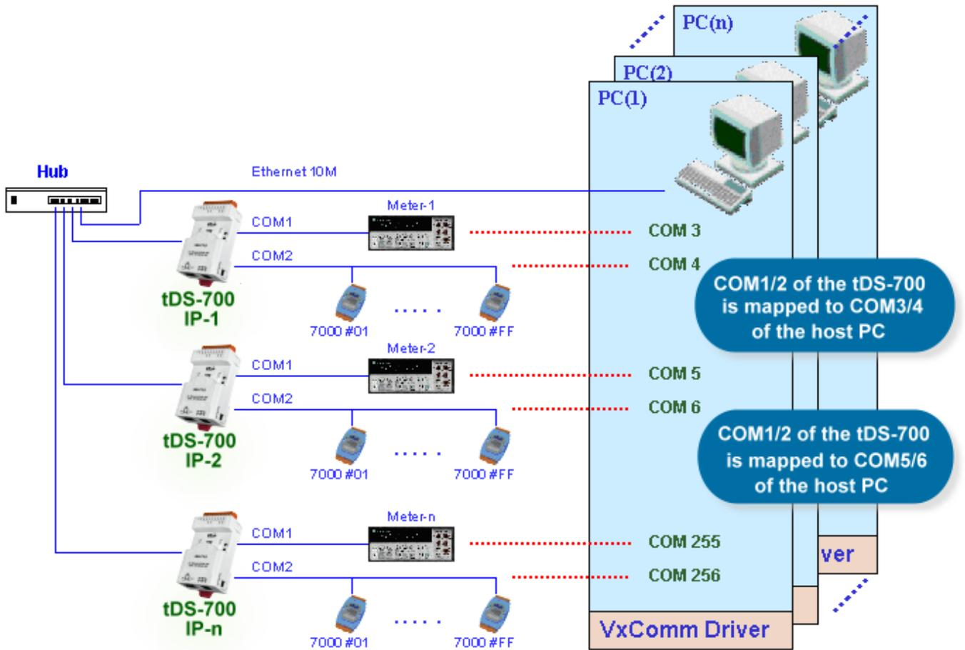
In the configuration above, Meter-1 is virtualized to link to COM3 of the host PC. Therefore, a program originally designed for the MS-COMM standard can access the meter without the need for any modification.
