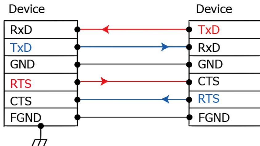
**Note:** FGND is the frame ground that is soldered to the metal shield on the DB-9 cable.
