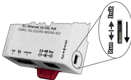
3. Connect both the tDS-700 and the Host computer to the same sub-network or the same Ethernet Switch, and then supply power (PoE or +12 to +48 VDC) to the tDS-700.
