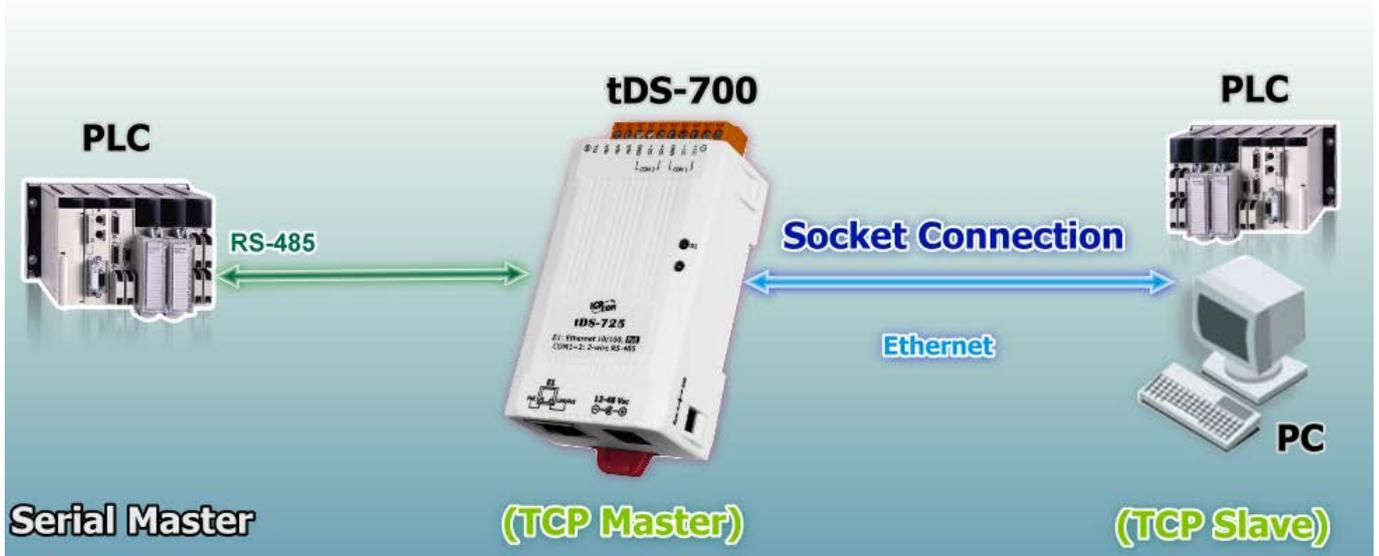
The following are examples of TCP Client Mode tests:
