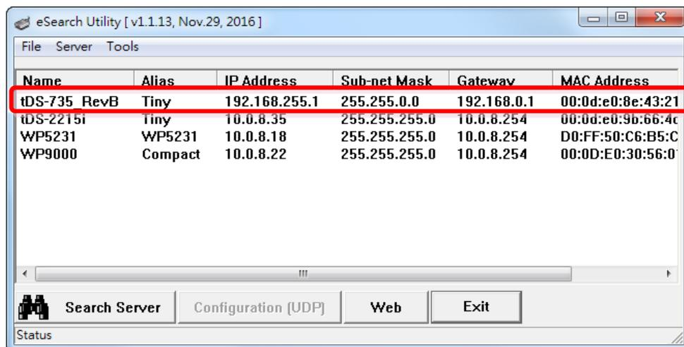
**Step 3** Double-click the name of the module to open the Configure Server (UDP) dialog box, and modify the basic settings as necessary, e.g., the IP, Mask and Gateway addresses, and then click the "OK" button to **save the new settings**.
