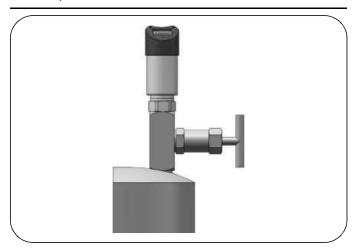
After the pressure in vessel is stable, slowly open the shut-off valve to start measuring.
