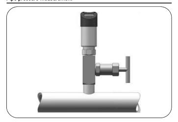
Can be installed with adapters on the pipe directly.
