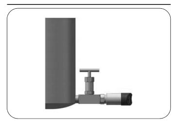
Can be used for liquid level measurement in open container. Media compatibility should be considered.
