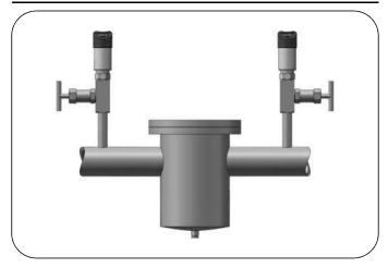
Two pressure switches can be used to create a differential measurement system, commonly used in the filter control or closed container level measurement.
