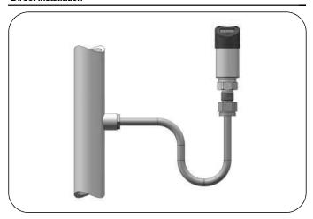
Light-weight pressure switch can be mounted directly on the pressure leading tube. When installing the maximum torque force can not exceed 50Nm.
