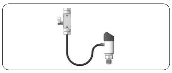
To safeguard against liquid media potentially traveling along the cable into the terminal box, the cable should be configured in a U-shape as shown, with the bottom of the "U" lower than the bottom of the pressure switch
