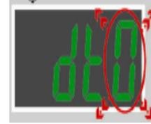
increment the latest digit (flashing) by pressing the **adjusting** key
