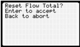
2. There is also an option to reset the flow totalizer using hardware: Short pins 14 and 15 of the probe connector.
