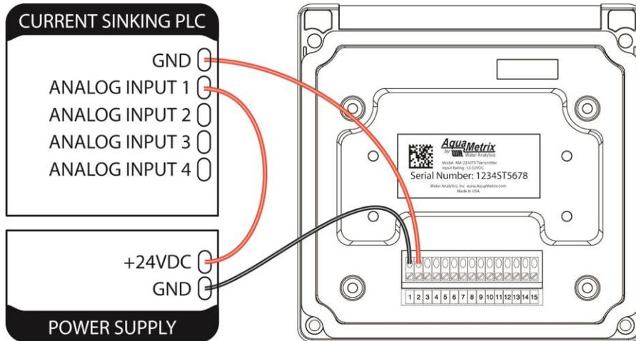
Figure 3-5 AM-2250TX with current sinking PLC
