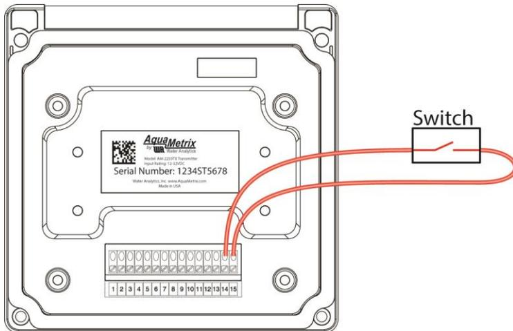
Figure 4-2 Flow Totalizer Reset using probe connector
