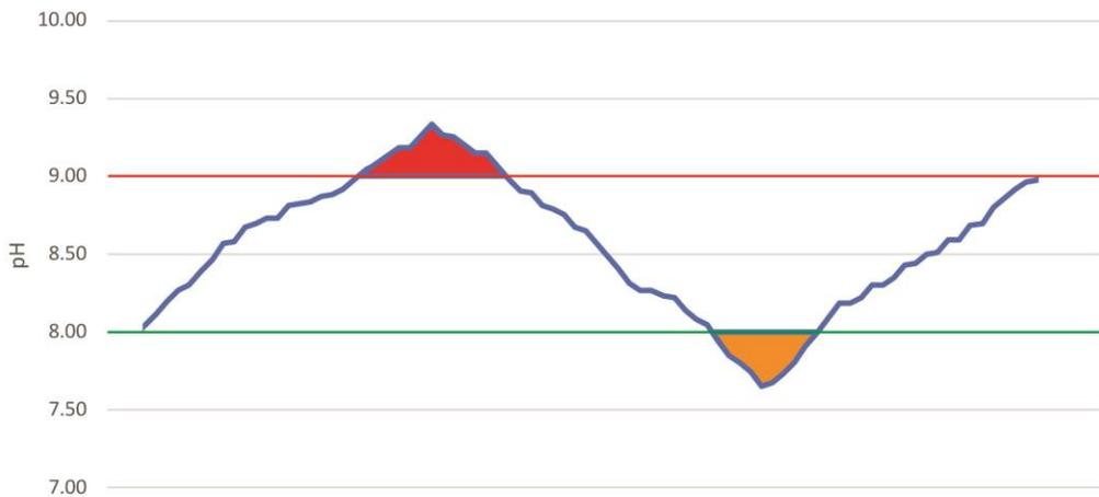
Figure 6-2 Example of pH control using relay.
