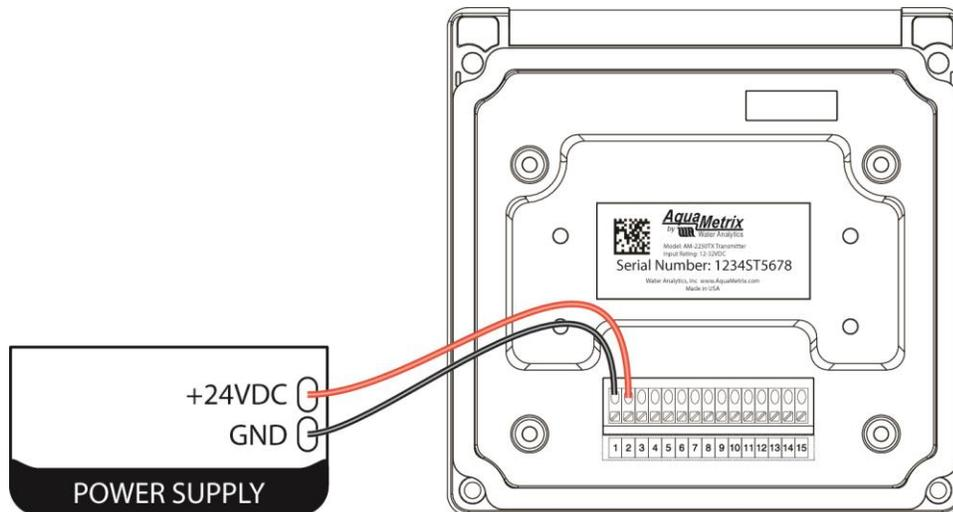
Figure 3-4 AM-2250TX wiring with external power supply.
