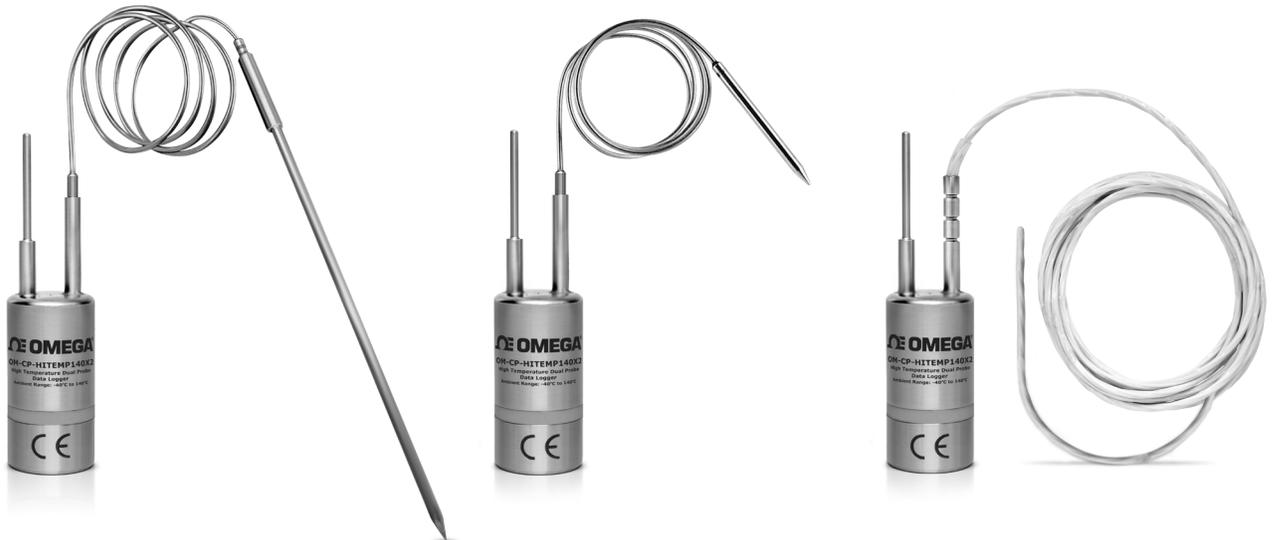
The OM-CP-HITEMP140X2-TD data logger models feature a 2" rigid transitional diameter probe to measure ambient temperature, combined with a second bendable or flexible probe option. The rigid 2" TD probe is made of stainless steel, offers an ultra-fast response time and is suitable for measuring ambient temperatures in the harshest environments.
