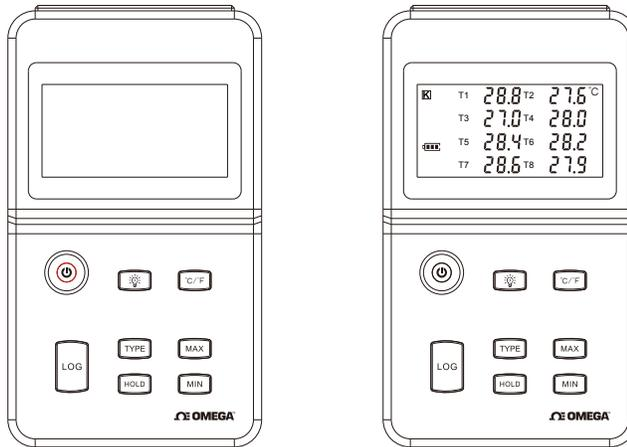
**Start Logging** - When the Logger is on and on stand-by (LCD does not have "LOG" logo display), press "LOG" button, LCD has "LOG" logo display, now the logger start logging and storing data.
