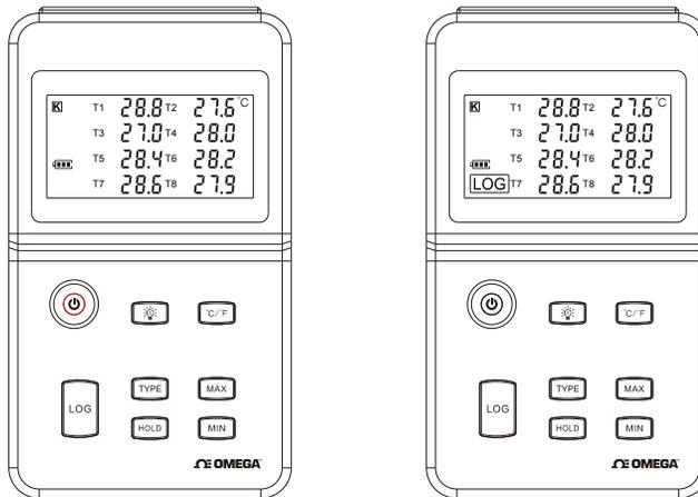
**Stop Logging** - When the Logger is on logging, long press "LOG", LCD display countdown time, loosen "LOG" button when countdown time finished, then the instrument switch from logging to standby state.
