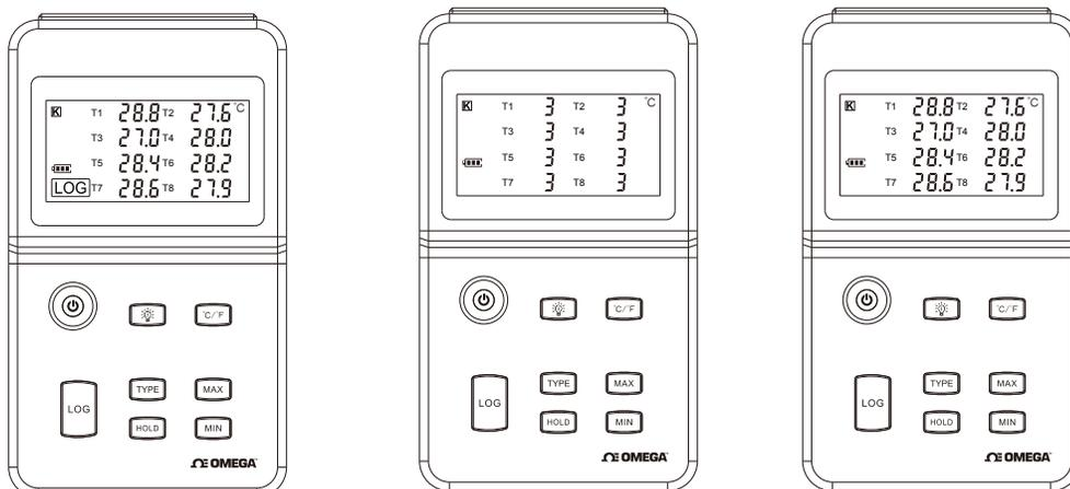
**Turn Off the Logger** - Push the "ON / OFF" Button for short pressing then LCD display is off.
