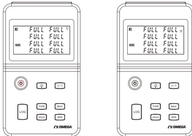
**Switchable °C or °F** - Press the "°C/°F" key shortly When instrument records data in degrees (the LCD displays the °C symbol), and the instrument switches to Fahrenheit as the recording unit display data (the LCD displays the °F symbol). It Can Switch back and forth between °C and °F as you Press this button repeatedly.
