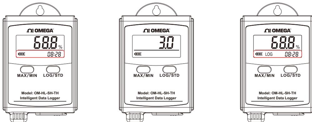
**Stop Logging** - When the logger is on logging, press "LOG/STD" for 3 seconds, LCD display time, loosen "LOG/STD" button when the LCD display "3.0", LCD does not have LOG logo display, then the logger will be on stand-by.
