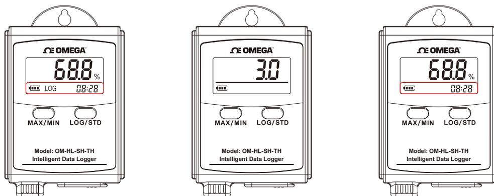
**Turn Off the Logger** - Push the“LOG/STD” Button for 5 Secs then LCD display is off.
