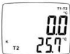
Every time the  $\overline{\text{T1-T2}}$  button is pressed and held, the main/secondary display position of T1 and T2 will be switched.
