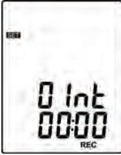
(2) Fig.2 Set interval time for data logging.
