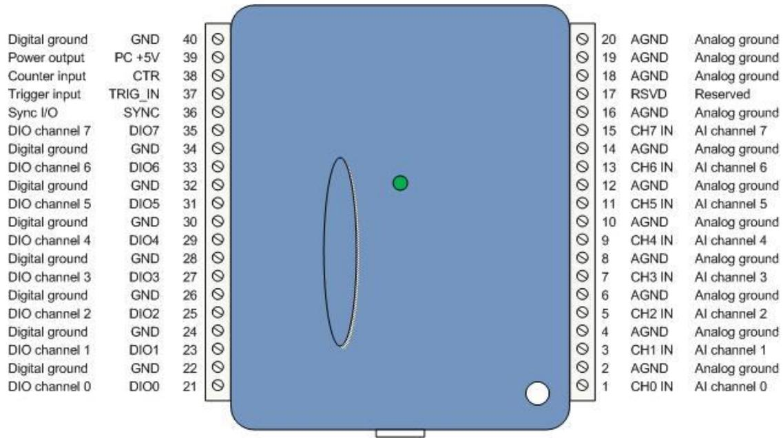
Figure 3. Screw terminal pinout
