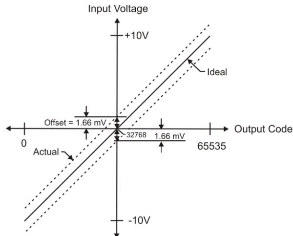
Figure 8. ADC transfer function with offset error
