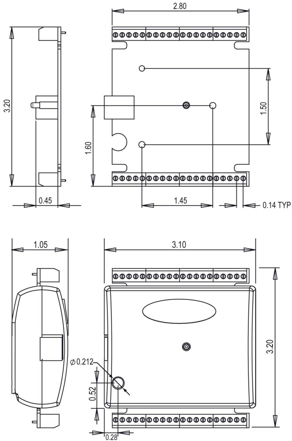
Figure 11. OM-USB-1608FS-Plus circuit board (top) and enclosure dimensions
