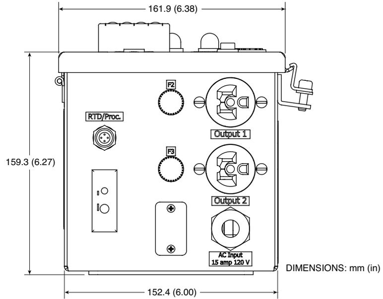
Figure 2-5. CNI-CB120SB Mounting Dimensions, Bottom View
