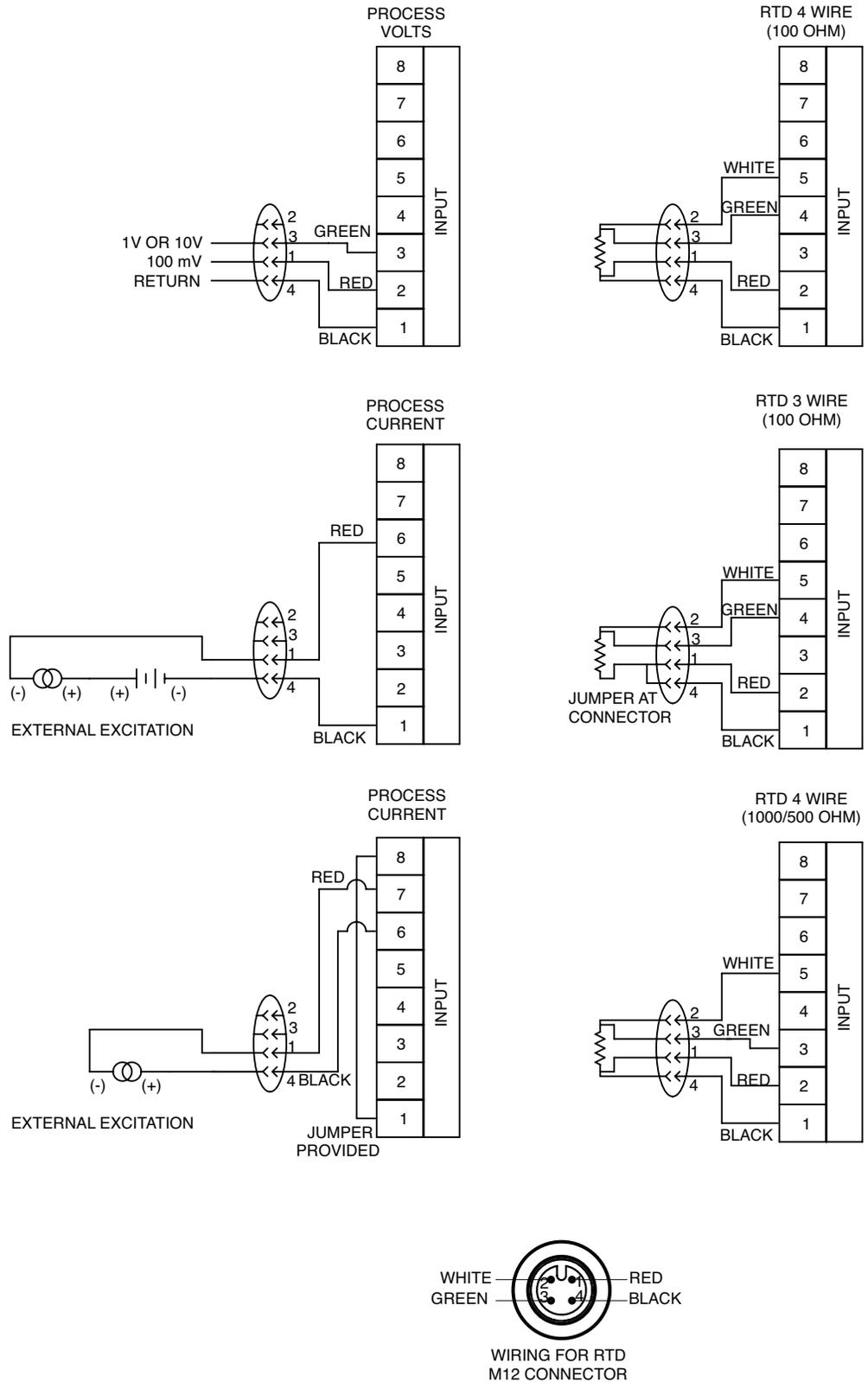
Figure 3-9. CNI-CB120SB Wiring Schematics
