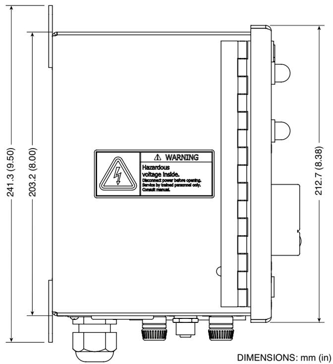
Figure 2-4. CNi-CB120SB Mounting Dimensions, Side View
