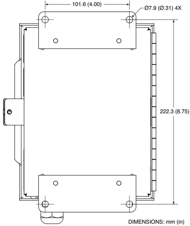
Figure 2-3. CNi-CB120SB Mounting Dimensions, Rear View
