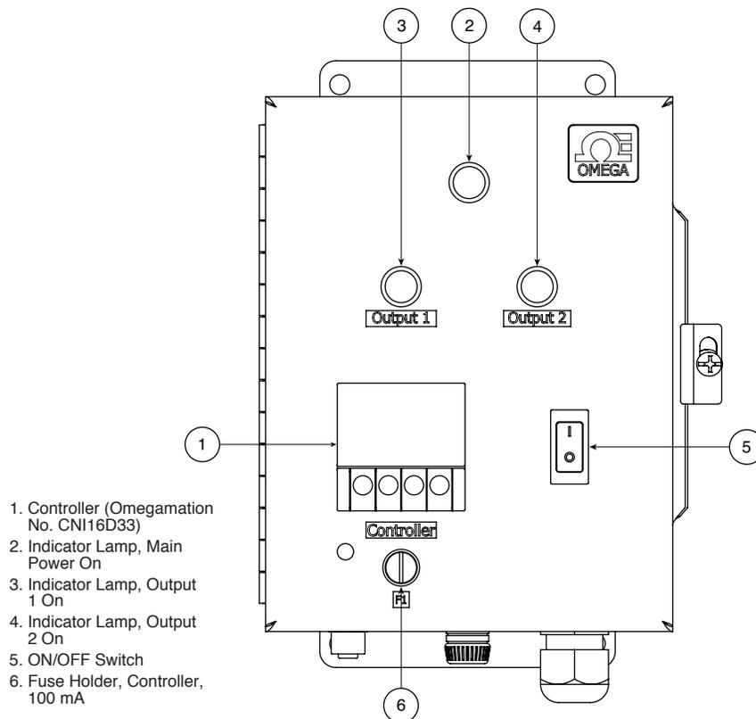
Figure 2-6. CNI-CB120SB Components, Front View (Closed)
