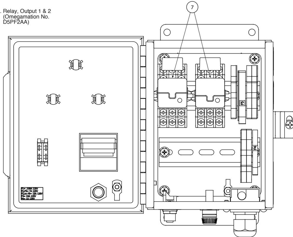
Figure 2-7. CNI-CB120SB Components, Front View (Open)
