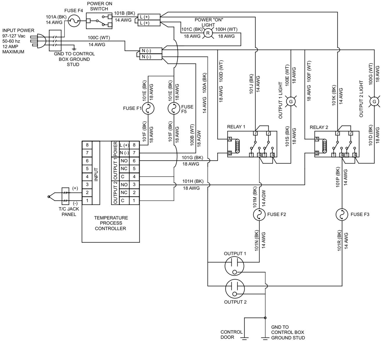
Figure 3-10. CNI-CB120SB Internal Wiring
