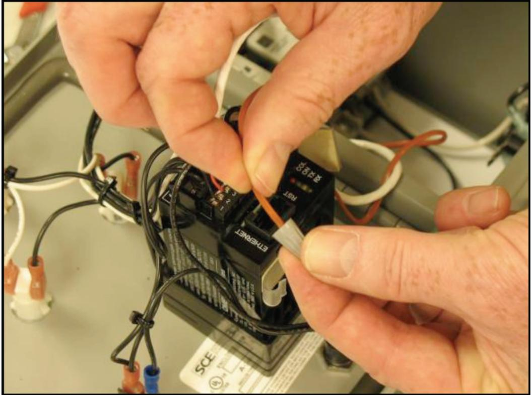
Figure 3-6. Place Wire Nut On T/C Wire
