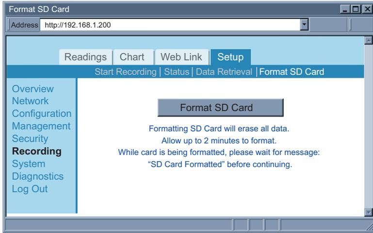
Figure 4.25 Recording Menu: Format SD Card
