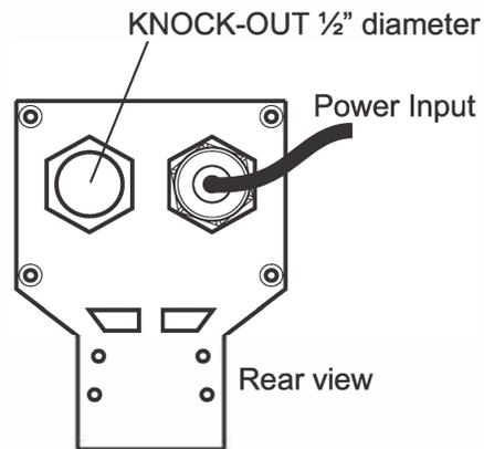
On panel or wall mounted units, wiring may be installed through the enclosure bottom or through the back panel. See below.
