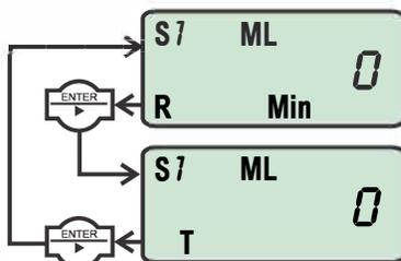
**FLOW RATE DISPLAY** - Indicates rate of flow, S1 = body size/range #1, ML = units displayed in milliliters, MIN = time units in minutes, R = flow rate displayed.
