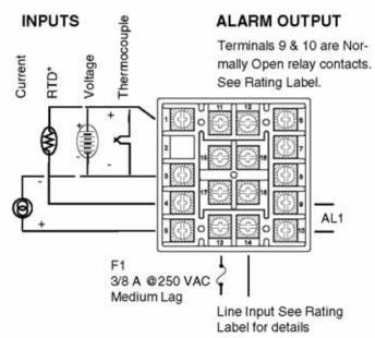
\* For 2-wire 1000  $\Omega$  RTD use terminals 1 & 3. For 2-wire 100  $\Omega$  RTD use terminals 1 & 3, and place a jumper wire between terminals 3 & 4.
