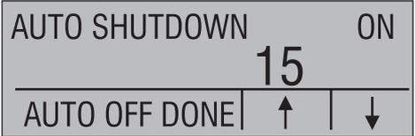
Use the AUTO OFF DONE option to set the parameters and return home. The auto shut off time is reset whenever a key is pressed.
