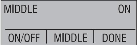
Use the DONE option to save the changes and return home. When a display is deactivated its configuration is retained. When the display is activated its configuration is checked against the configurations of the other currently active displays, if the configurations are in conflict the recalled display's configuration is modified to avoid the conflict. If all three displays are deactivated the LOWER display will come on automatically.
