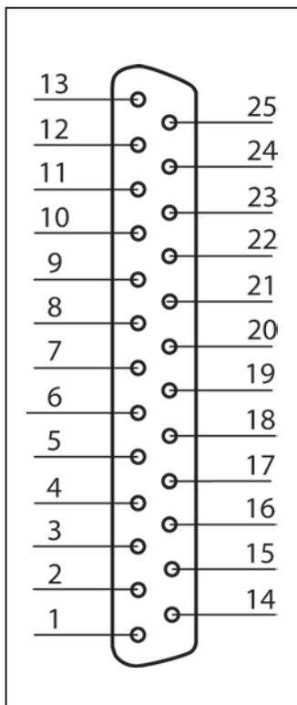
**FIGURE b-2, FMA6500 25 PIN "D" CONNECTOR CONFIGURATION**
