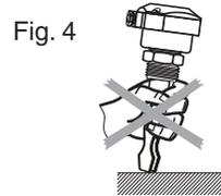
When cleaning the Forks use a soft brush to ensure that the coating or polishing is not damaged or scratched.
