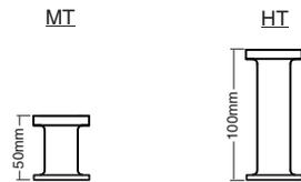
Extended necks for medium temperature (up to 100°C) and high temperature (up to 120°C)
