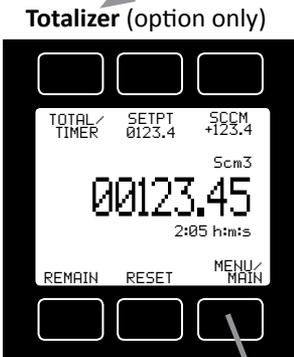
If your controller was ordered with the **Totalizer** option (page 52), pushing the **TOTAL** button once will bring up the **Totalizing Mode** display. Pushing **MENU** will bring up the **Select Menu** display.
