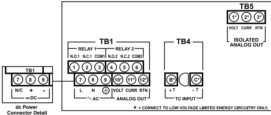
**Figure 5-3. Connector Label (AC-Powered and DC-Powered Detail)**
