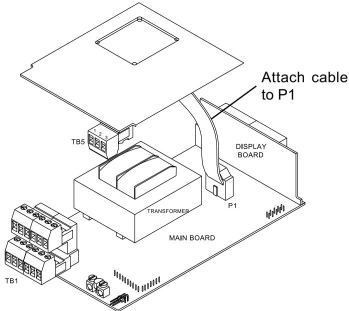
**Figure 7-7. Isolated Analog Output Upper Board Installation**
