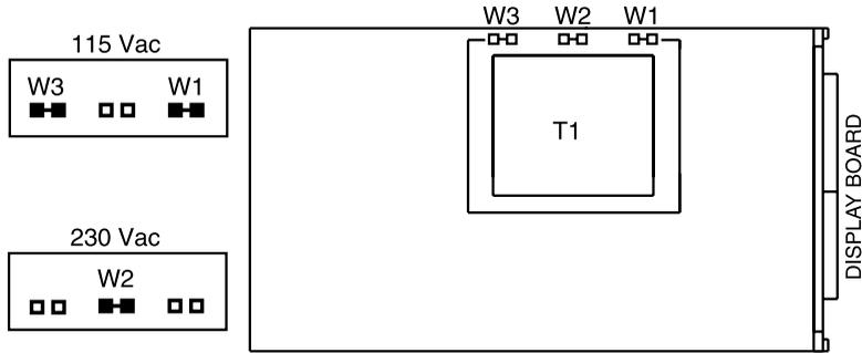
**Figure 6-1. Main Board Power Jumpers (W1, W2, W3)**
