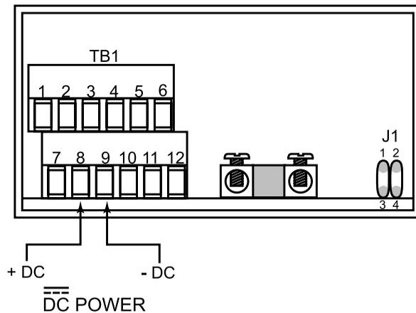
**Figure 7-3. Main Power Connections - DC Powered Unit**
