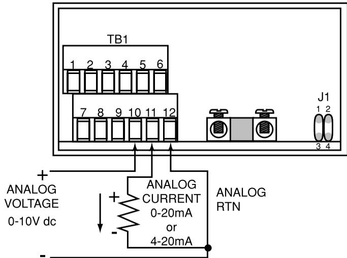
**Figure 7-4. Analog Output Connections**
