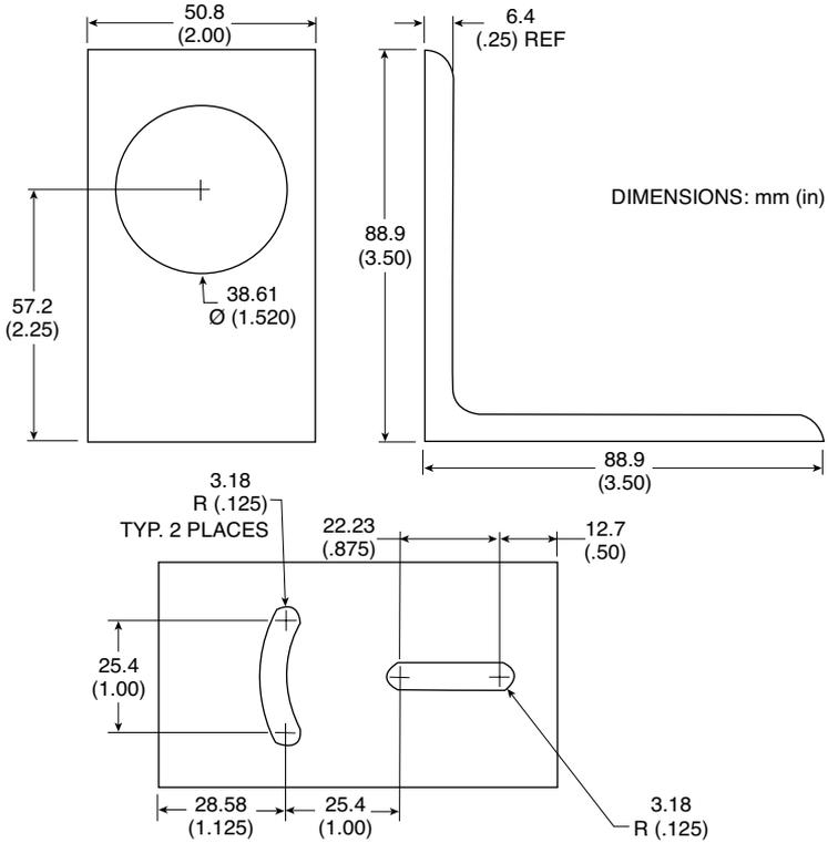
Fig. 2-4. Mounting Bracket Dimensions
