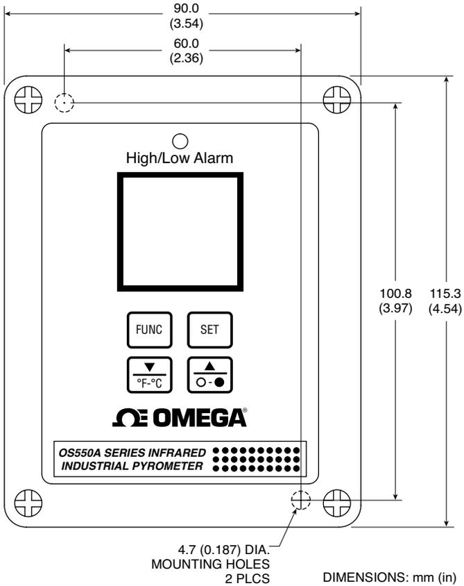
Fig. 2-2A. Aluminum Housing Dimensions
