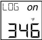
The thermometer can log temperature data in real time. The logged data is stored in the non-volatile memory, so removing the power will not affect or erase the data. The data is logged based on the data recording interval (PRN) which can be set anywhere from 1 to 1999 seconds. The thermometer can log up to 800 data points. Therefore, the logging period can be anywhere from 13 minutes (1 second recording interval) up to 18.5 days (1999 second recording interval). To log temperature in real time:
