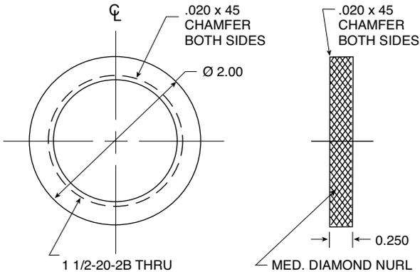
Fig. 2-5 Mounting Nut Dimensions
