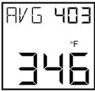
is the true average temperature since the temperature measurement session starts. The average temperature under continuous operation is accurate for a limited period of time (refer to the specifications). However, the AVG temperature function can be used indefinitely when the thermometer is operating intermittently.
