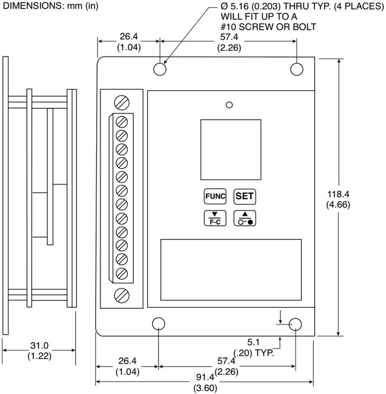
Fig. 2-3. OEM Style Main Display with Mounting Plate
