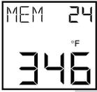
The thermometer can store up to 800 temperature data points on command. This data is stored in the non-volatile memory, so removing power will not affect or erase this data. To store temperature data:
