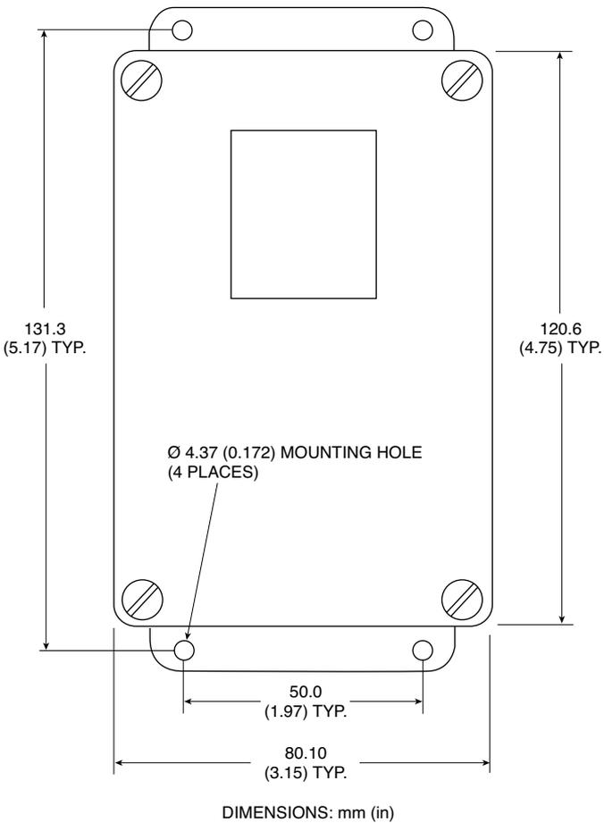
Fig. 2-2. Plastic Housing Dimensions
