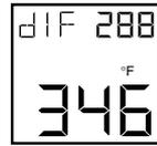
is the difference between the MAX and MIN temperatures.
