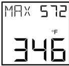
is the maximum temperature since the temperature measurement session starts (pulling the trigger).
