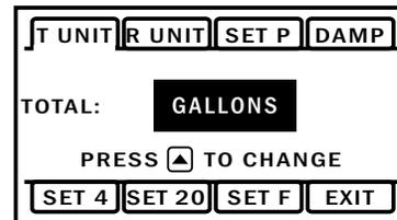
**Select a new setting.** Select the new setting by scrolling through a list of selections as in the screen illustration below by tapping the left button to find a different TOTAL unit.
