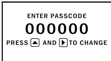
The default passcode is 000000. If a different passcode has previously been set, then the user must enter that passcode at this time. After entering the passcode, or leaving it at 000000 if using the default passcode, the user does the tap and hold sequence to move into the menu system.
