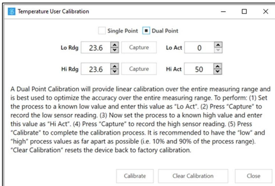
Figure 18: SYNC Configuration Software – Dual Point Calibration
