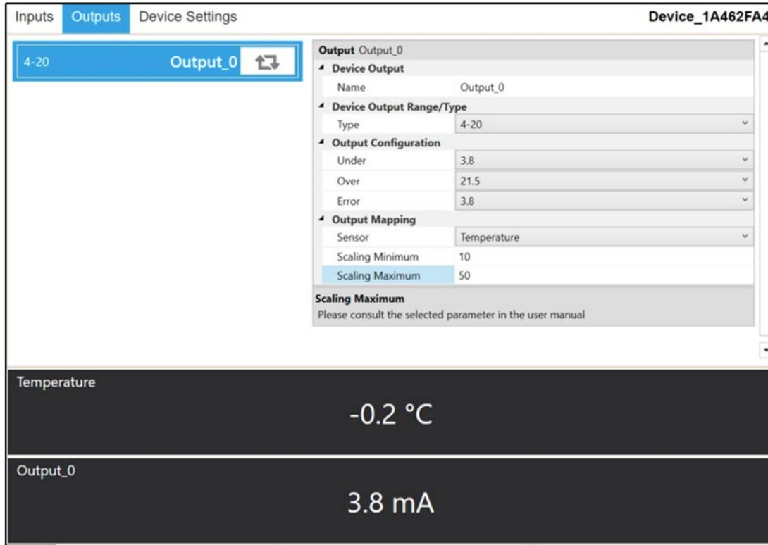
Figure 27: SYNC Configuration Software – 4-20 mA Output Sensor Mapping
