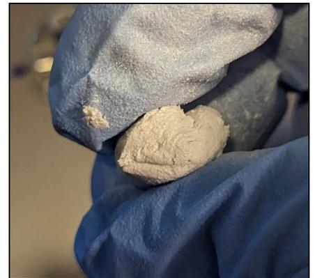
Figure 9: Thoroughly mix the epoxy
