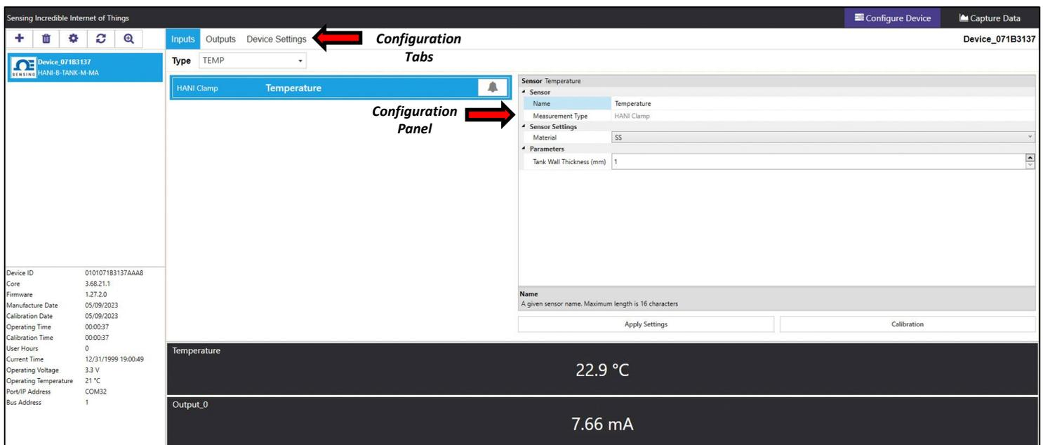
Figure 16: SYNC Configuration Software – HANI™ User Interface
