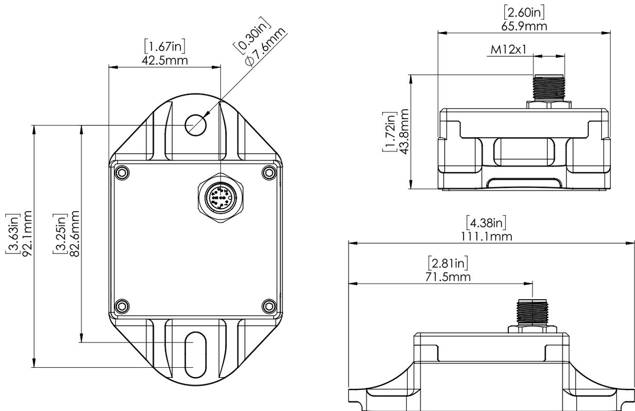
Figure 1: HANI™ Tank Sensor Mechanical Dimensions in Inches
