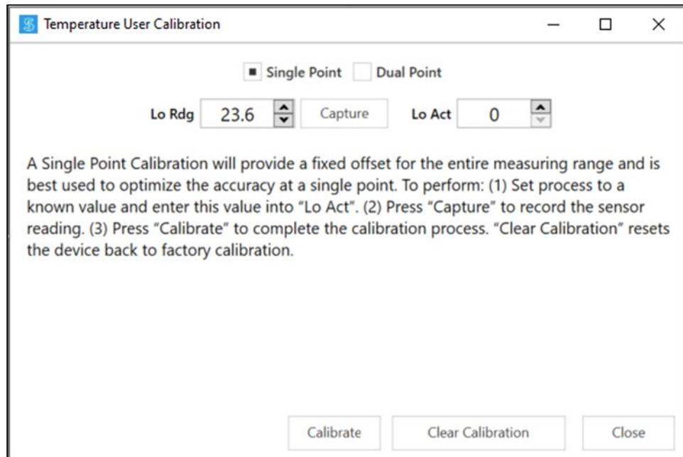
Figure 17: SYNC Configuration Software – Single Point Calibration
