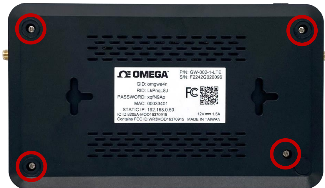
Figure 53: GW-002 Device Screws
