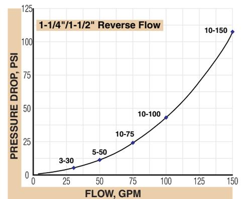
The pressure drop curves are valid for fluids with density and viscosity similar to factory test fluids. Fluids, especially with higher viscosity than these test fluids, will yield a higher pressure drop through the flow meter and piping system per a given flow volume.
