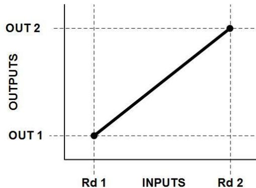
**Figure 11. Output Scaling**
