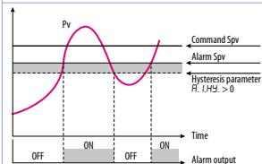
Upper deviation alarm value of alarm setpoint less than "0" and hysteresis value greater than "0" (Par.128 R.I.HY > 0).
