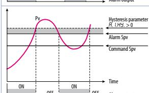
Lower deviation alarm value of alarm setpoint less than "0" and hysteresis value greater than "0" (Par.128 R.I.HY > 0).
