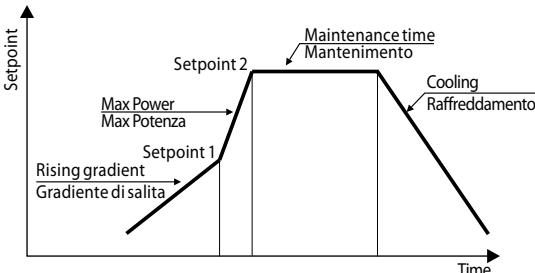
Cycle starts at each activation of the controller, or via digital input if it is enabled for this type of functioning (parameters 231, 239, 247, 255 set as 5E./5E. or P.M.).
