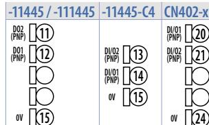
Digital output PNP (including SSR) for command or alarm.
