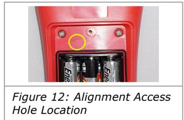
*Figure 12: Alignment Access Hole Location*
