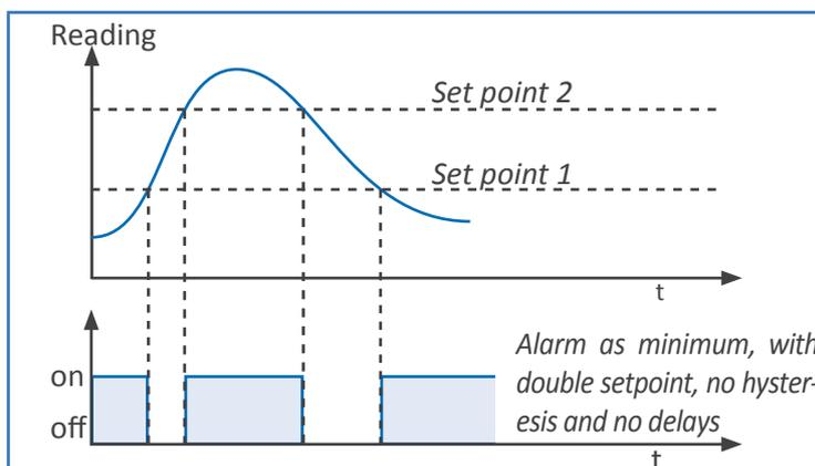
Figure 8 - Example of alarm with double setpoint
