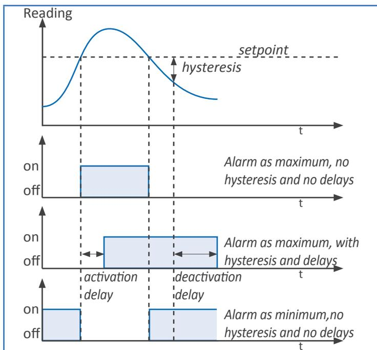
Figure 6 - Examples of alarms with 1 setpoint
