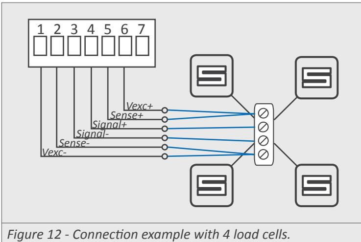
Figure 12 - Connection example with 4 load cells.
