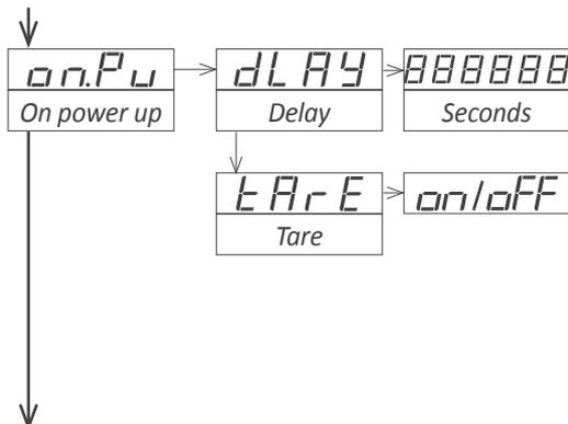
The 'On power up' ('on.Pu') menu assigns functions to apply when the instrument restarts after a power loss. See section 1.12.14 for additional information.
