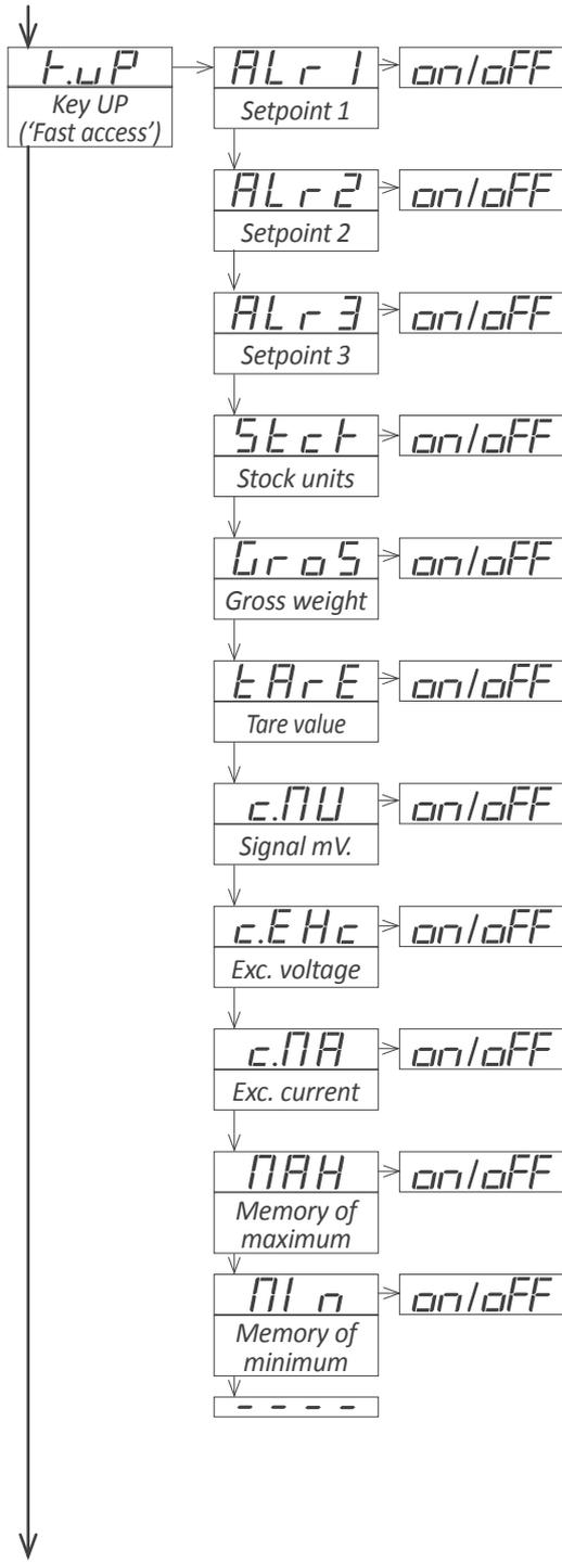
At the 'Key UP (fast access)' ('K.uP') menu configure which functions and parameters will be accessible through the 'fast access' menu. Select 'on' to activate each function. See section 1.12.13 for additional information.
