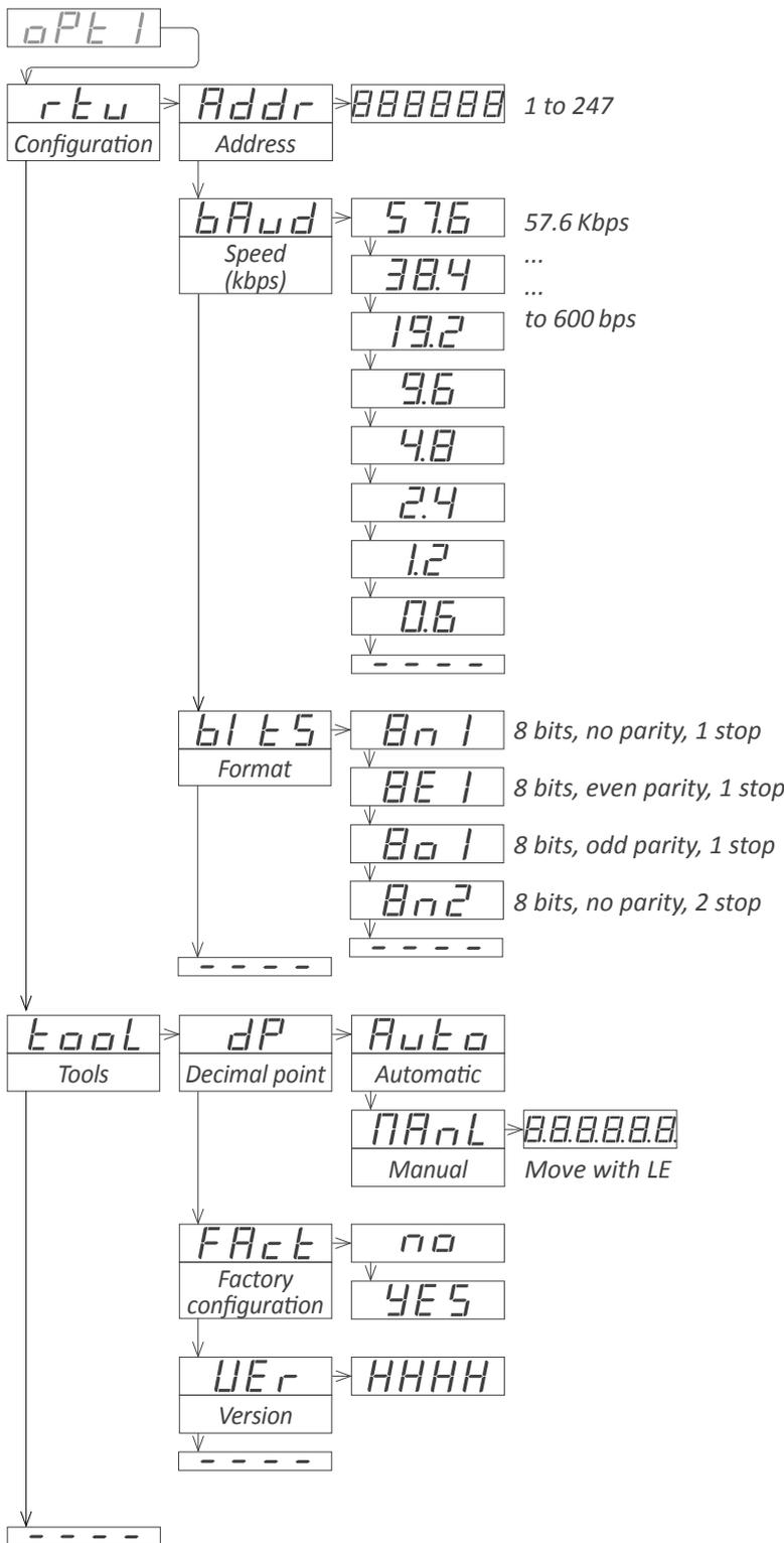
Configure at menu 'Configuration' ('rtu'), the address value between '1' and '247' at parameter 'Address' ('Addr'), bus speed in kbps at parameter 'Speed' ('bAud') and data format at parameter 'Format' ('bltS').
