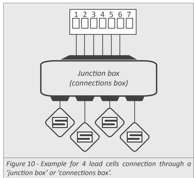
Figure 10 - Example for 4 load cells connection through a 'junction box' or 'connections box'.
