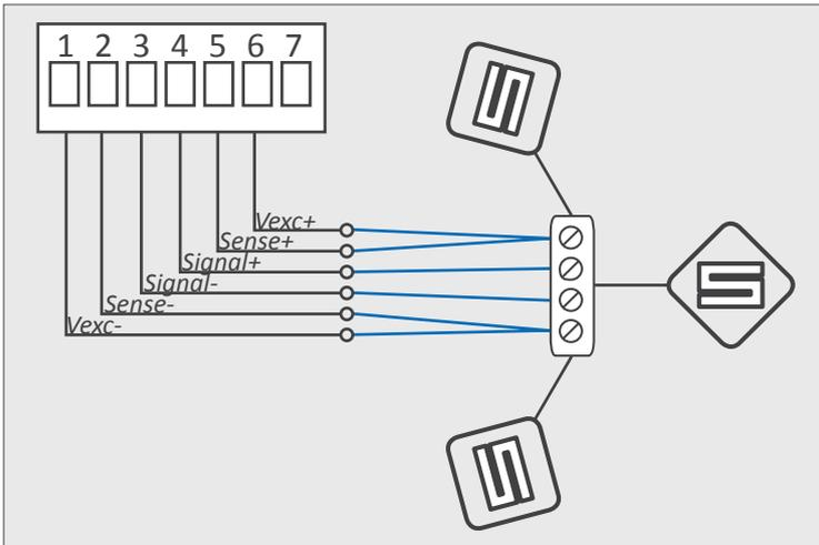
Figure 11 - Connection example with 3 load cells.
