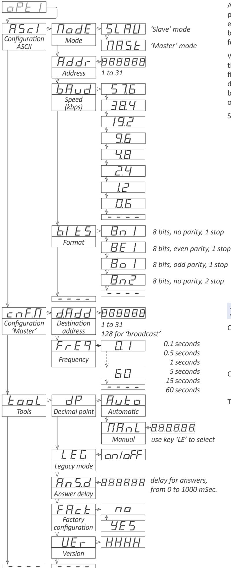
At menu 'Configuration ASCII' ('ASCI'), configure the instrument at parameter 'Mode' ('ModE') to work as 'slave' or 'master', at parameter 'Address' ('Addr') set the address value from '1' to '31', set the bus speed in kbps at parameter 'Speed' ('bAud') and set the data format at parameter 'Format' ('bltS').
