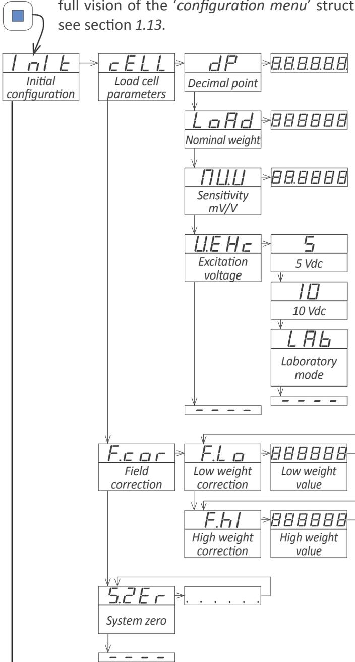
At the initial set up of the instrument, first configure the theoretical part of the load cell at the 'Load cell parameters' ('cELL') menu and later configure the empirical part of the load cell at the 'Field correction' ('F.cor') menu. See section 1.12.2 for additional information.
