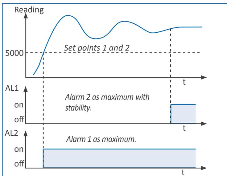
Figure 7 - Example of alarm with stability
