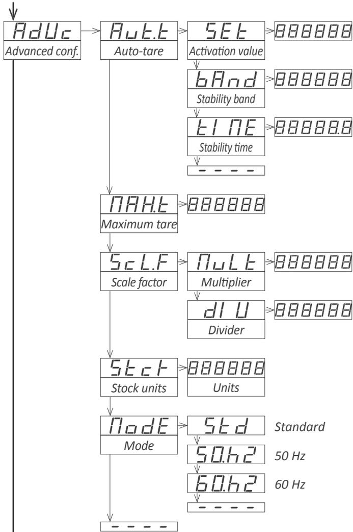
At the 'Auto-tare' ('Aut.t') menu configure the activation value and stability values to control the automatic activation of the tare, when weight is removed from the cell. See section 1.12.4 for additional information.
