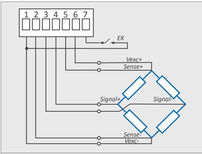
Figure 4 - Example for connections with 1 load cell.
