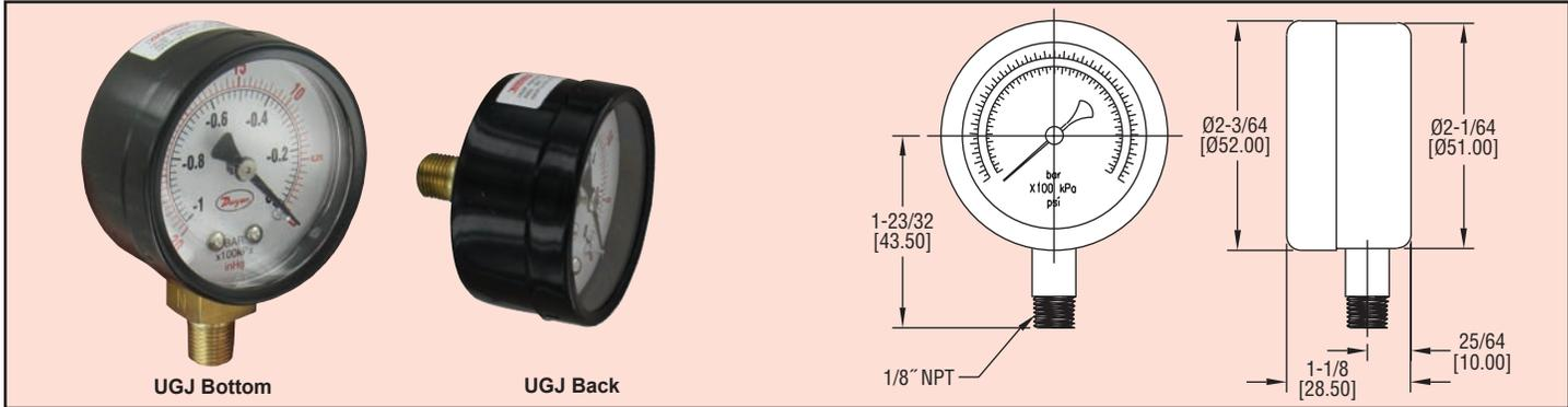
The Series UGJ Utility Gages possess dual psi and bar (x100 kPa) scales with 2.5% accuracy. The 2" UGJ gages are designed with black steel housings. Wetted parts include a brass socket and phosphor bronze tube. A wide offering of ranges are available from full vacuum to 300 psi.
