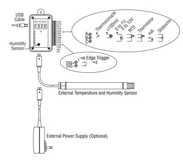
Having selected the correct sensor type, the appropriate connections can be made. The type of sensor used must be selected via the software prior to issue.
