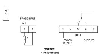
**Probe Range:** PTC: -58 to 302°F (-50 to 150°C); NTC: -58 to 230°F (-50 to 110°C). **Input:** PTC (1000 Ω @ 25°C) or NTC (10 KΩ @ 25°C) thermistor. **Output:** SPDT relay rated 16 A @ 240 VAC resistive, 10 FLA, 60 LRA. **Horsepower Rating (HP):** 1 HP. **Control Type:** On/Off.
