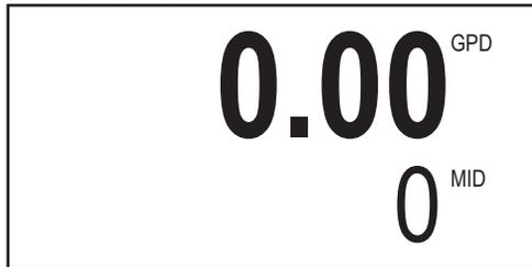
The HOME Screen, shown above, is the normal screen which displays TOTAL flow volume and flow RATE. The Four buttons below the LCD display are used to access menu screens for viewing and changing setup parameters.
