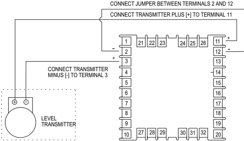
**Figure 3: Transmitter wiring**
