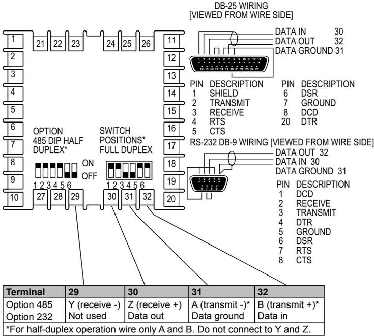
**Figure 4: Wiring for options**
