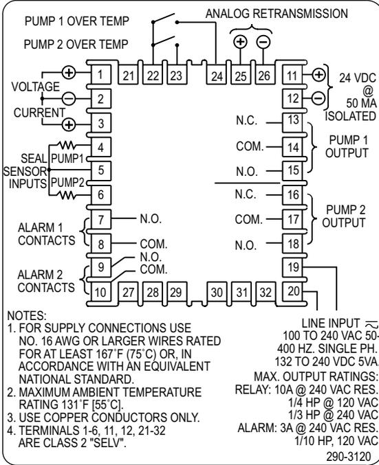
**Figure 2: Wiring**
