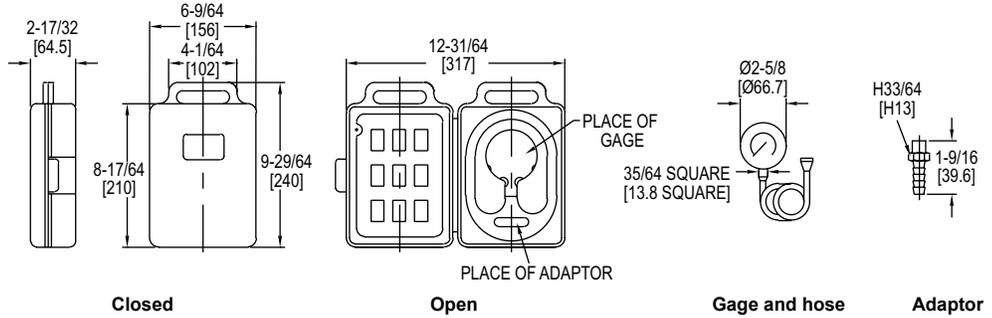
The **Series LPTK Gas Pressure Test Kit** is ideal for testing LP and natural gas lines and controls. The kit's gage shows if proper pressure is present or if a leak exists. Series LPTK is easier to use than a manometer and includes a sturdy case for added durability and safe handling.
