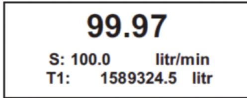
Figure 4 - Initial PI Screen (Flow Controller)
