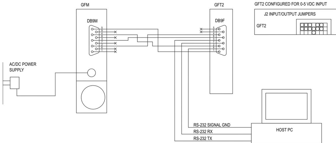
Figure 34: Connecting GFT2 to the GFM using 5 to 10 VDC output from DB9 connector.
