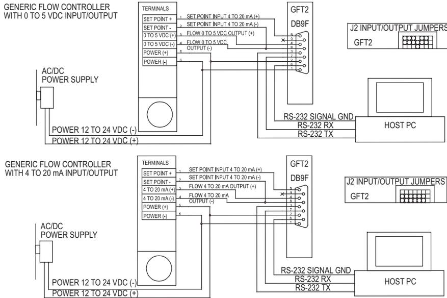
Figure 39: Connecting GFT2 to the Generic Flow Controller
