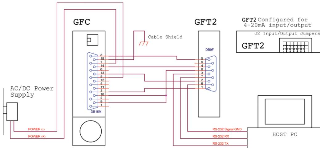
**Figure 36: Connecting GFT2 to the GFC Using 4 to 20 mA Input/Output from DB15 Connector.**
