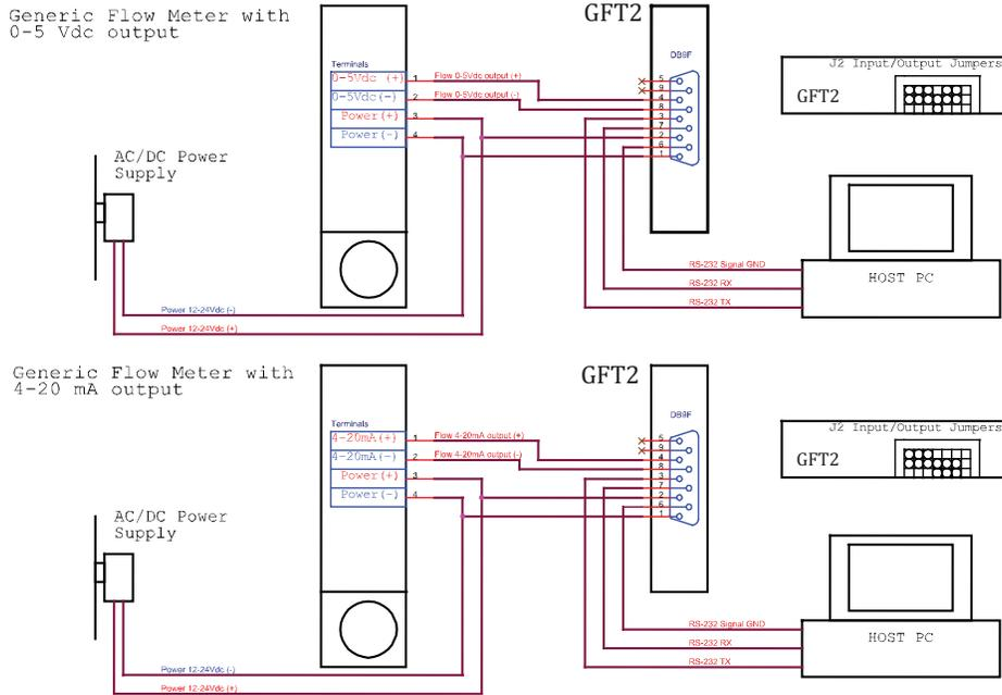
Figure 38: Connecting GFT2 to the Generic Flow Meter
