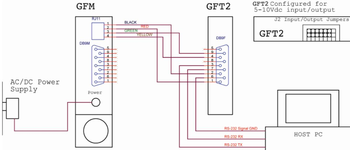
Figure 33: Connecting GFT2 to the GFM using 5 to 10 VDC output from RJ11 connector.
