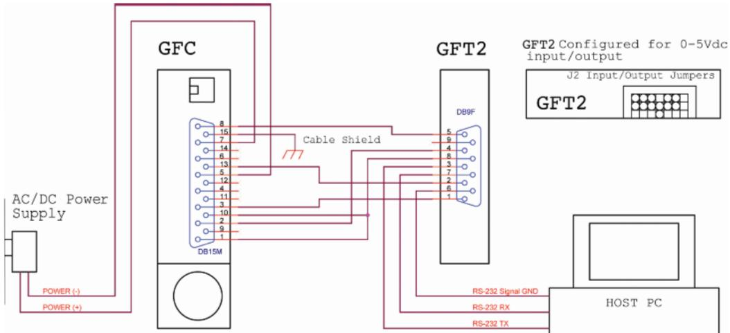
**Figure 35: Connecting GFT2 to the GFC Using 0 to 5 VDC Input/Output from DB15 Connector.**
