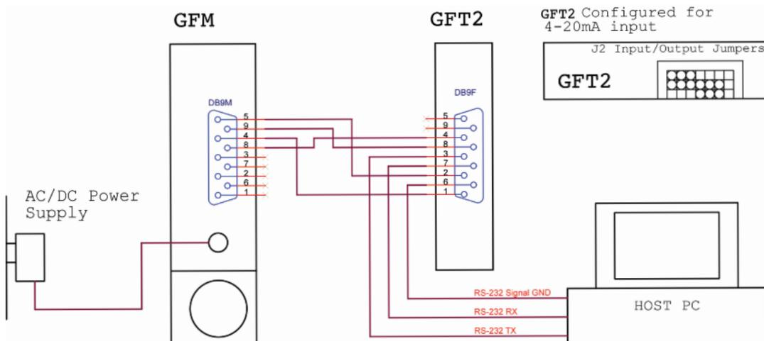
Figure 32: Connecting GFT2 to the GFM using 4-20mA output from DB9 connector.
