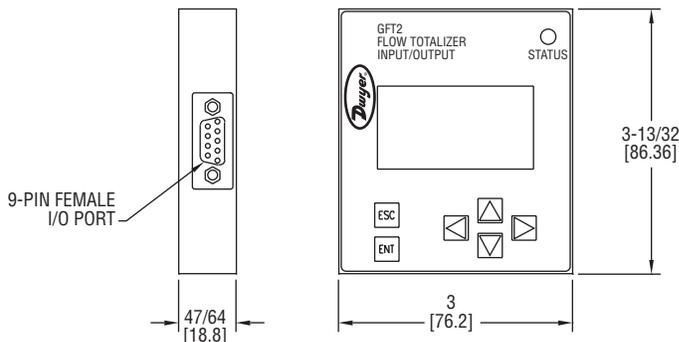
The Series GFT2 Flow Totalizer is a microcontroller driven device designed to linearize the flow meter and controller flow curve plus display the instantaneous flow rate, total, and accumulated total. The totalizer is intended to be used with analog flow meters and controllers with analog 0 to 5 VDC, 0 to 10 VDC, or 4 to 20 mA interface. RS-232 or RS-485 digital interface is available.
