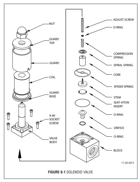
Various corrosive gases may demand more frequent replacement of VITON<sup>®</sup> O-rings and seals inside the valve. Be sure to use an elastomer material, appropriate for your specific gas application. Contact your distributor or Dwyer for optional sealing materials available.
