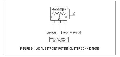
It is recommended that a potentiometer between 5K to 10K ohm and capable of at least 10-turns or more for adjustment be used. Use the control potentiometer to command the percentage of flow desired.
