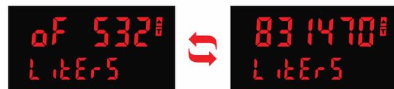
In the diagrams above, the flow totalizer is displaying 532,831,470 by toggling between a display of “oF 532” and “831470”. Notice the T with arrow ▲ symbol is lit up indicating the display is in overflow mode.
