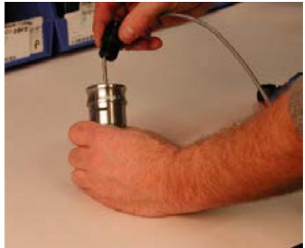
*1. Remove Strain Relief from the PDWS Series Meter*
