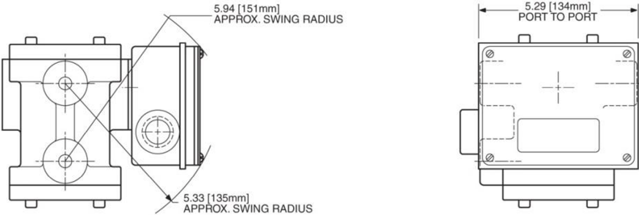
Figure 26: Vane/Piston H0 - Transmitter with HART PI, LL, LP, and LH dimensions
