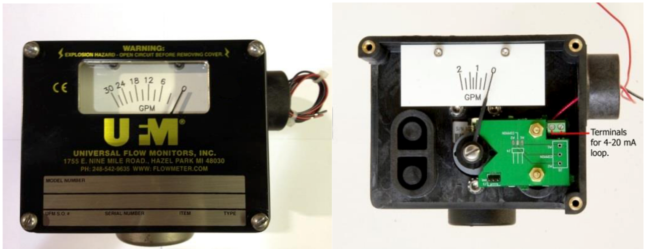
Figure 4: Terminals for 4 to 20 mA loop
