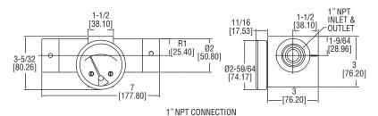
The Series DTFO Variable-Area Flowmeter for Oil measures oil rates with ±2% of full-scale accuracy at an affordable price. Durable metal construction ensures great compatibility and the strength to withstand system pressures of up to 3000 psig (200 bar). With a wide variety of flow ranges available, the Series DTFO can be used with many different applications all at an economical price.
