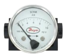
The Series DTFA Variable-Area Flowmeter for Gases measures gas rates with  $\pm 5\%$  of full-scale accuracy at an affordable price. Rugged aluminum construction ensures great compatibility and the strength to withstand system pressures of up to 3000 psig (200 bar). With a wide variety of flow ranges available, the Series DTFA can be used with many different applications all at an economical price.
