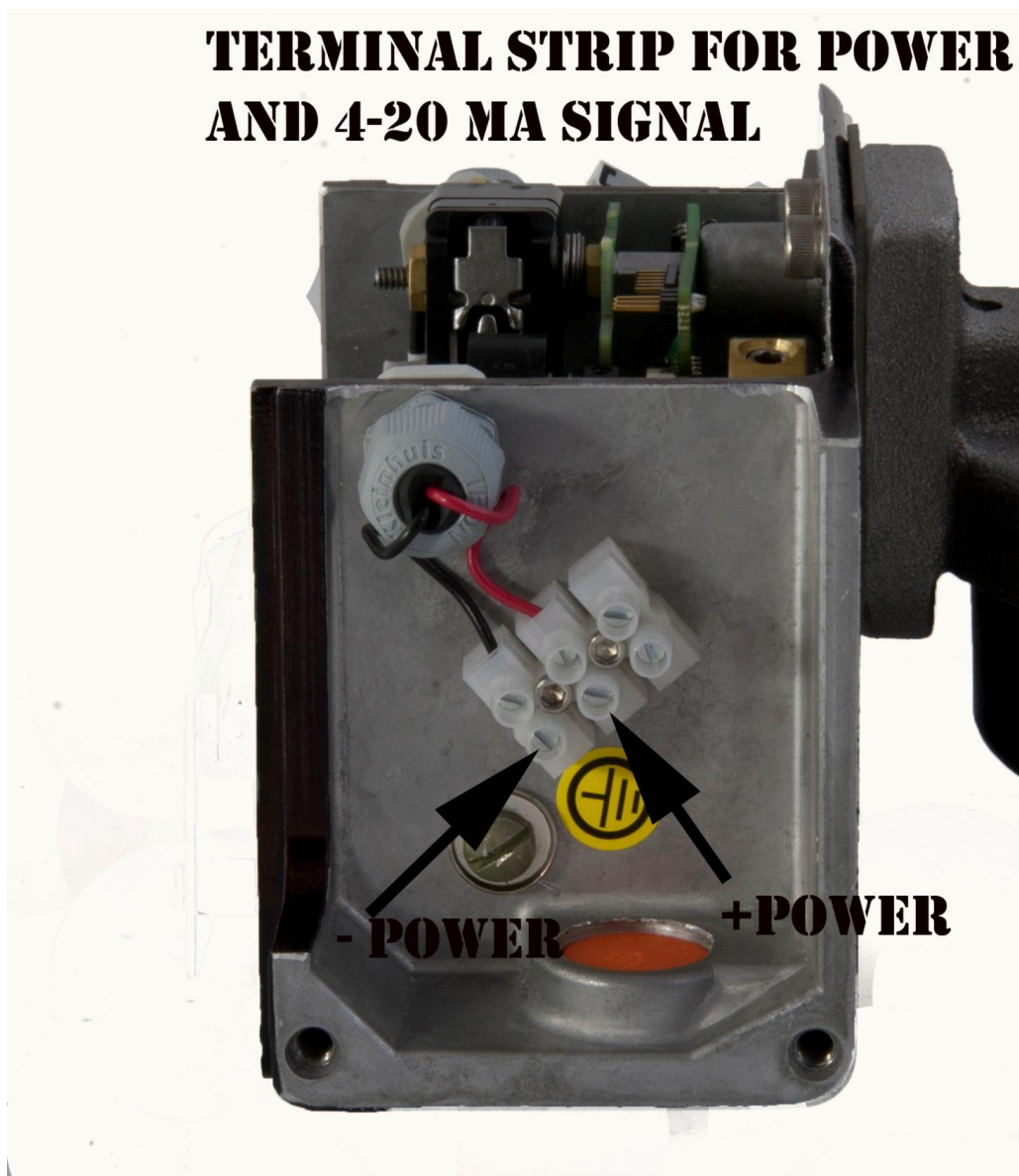
Figure 32: Terminal Strip for Power and 4-20 mA Signal
