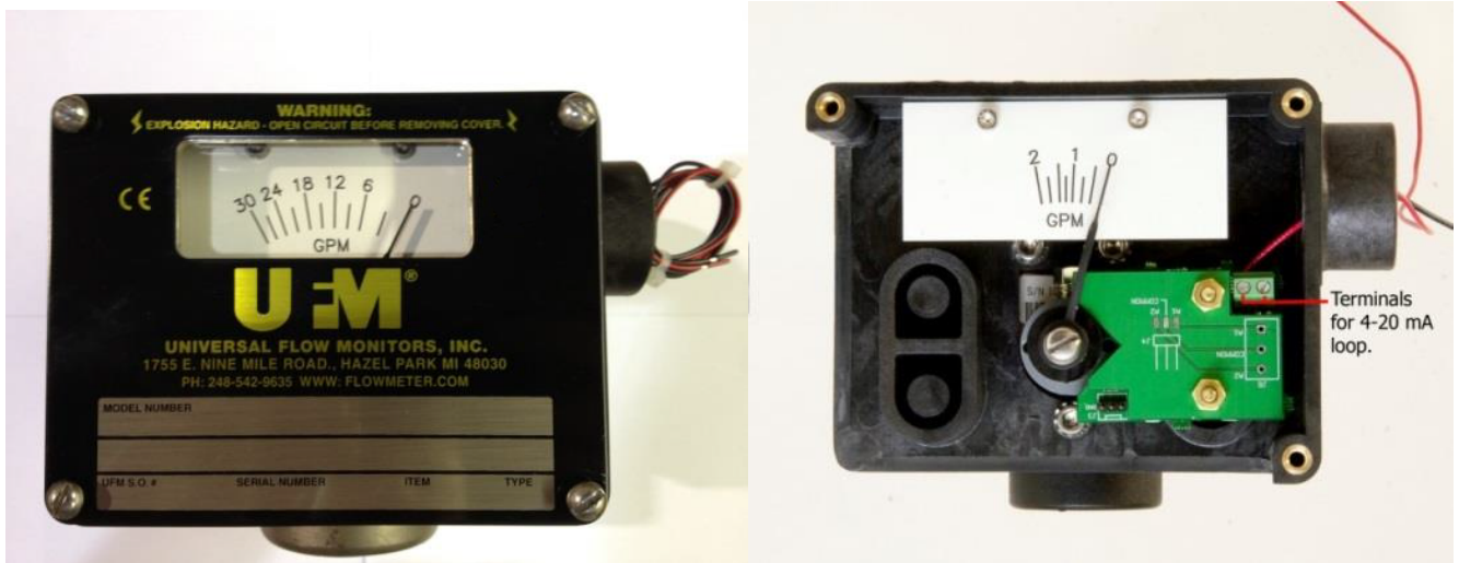
Figure 6: Terminals for 4-20 mA loop
