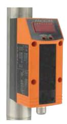
The Series CAM Compressed Air Meter operates by the calorimetric measuring principle to detect the standard volume flow of operating compressed air. It is designed specifically to evaluate the current flow rate and the current consumed quantity in compressed air systems. With an easily programmable digital display, this unit offers a quick, accurate readout. The Series CAM is constructed of high-grade materials and is virtually maintenance free.
